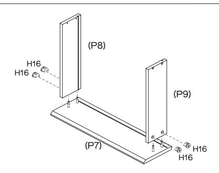
Insert 4 x Small Cam Nuts (H16) into the holes of Small Drawer Sides (P8, P9). Rotate the cam nuts so the arrows point towards the incoming cam bolts. Push Small Drawer Sides (P8, P9) into place and tighten the cam nuts.
