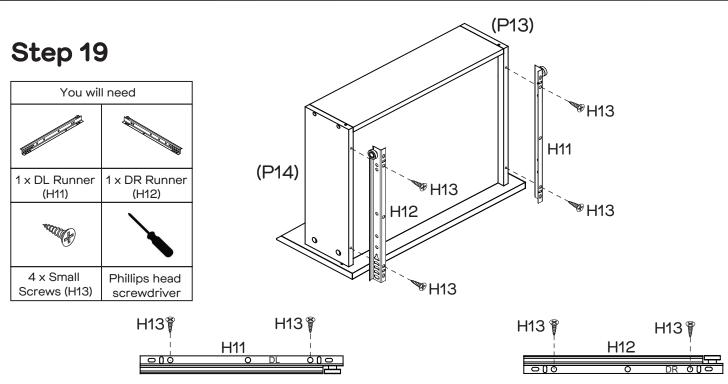
Attach 1 x DL Runner (H11) to the bottom of Left Drawer Side (P13) and 1 x DR Runner (H12) to the bottom of Right Drawer Side (P14) with  $4 \times 5$  Small Screws (H13).
