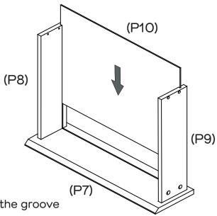
Slide Small Drawer Base (P10) into the groove in Small Drawer Sides (P8, P9).
