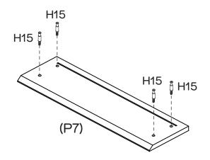
Attach 4 x Small Cam Bolts (H15) into Small Drawer Front (P7).
