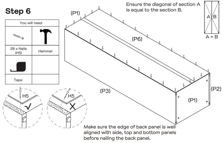
Attach Back Panel (P6) to the cabinet with 28 x Nails (H5) using hammer. Please measure with a tape to ensure that the spacing of the nails is consistent, and make sure the tip of the nails are vertically centered on the edge of the Side Panels(P2, P3) and Top/Bottom Panels (P1).
