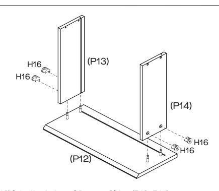
Insert 4 x Small Cam Nuts (H16) into the holes of Drawer Sides (P13, P14). Rotate the cam nuts so the arrows point towards the incoming cam bolts. Push Drawer Sides (P13, P14) into place and tighten the cam nuts.
