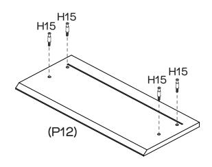
Attach 4 x Small Cam Bolts (H15) into Drawer Front (P12).
