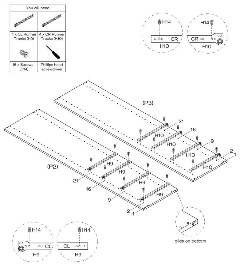
Attach 4 x CL Runner Tracks (H9) to Left Side Panel (P2) with 8 x Screws (H14). Attach 4 x CR Runner Tracks (H10) to Right Side Panel (P3) with 8 x Screws (H14).
