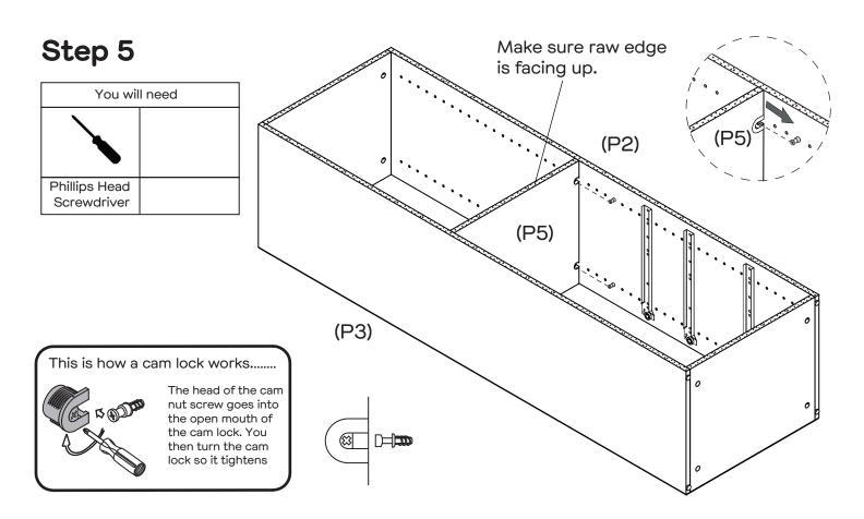
Adjust the opening of cam locks is facing the cam nut screws, then push Shelf Panel (P5) into place and tighten the cam locks.
