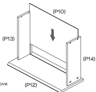
Slide Drawer Base (P10) into the groove in Drawer Sides (P13, P14).
