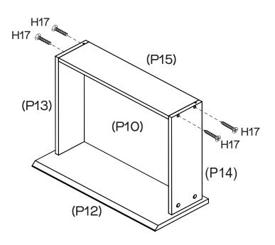
Attach Drawer Back (P15) to Drawer Sides (P13, P14) with 4 x Long Screws (H17), make sure that the groove lines up the whole way around the drawer.
