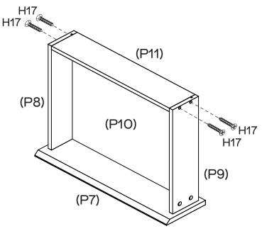
Attach Drawer Back (P11) to Small Drawer Sides (P8, P9) with  $4 \times 1$  Long Screws (H17), make sure that the groove lines up the whole way around the drawer.
