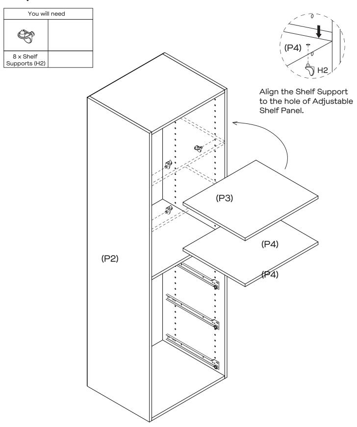
Insert 8x Shelf Supports (H2) into the holes of Side Panels (P2, P3) as shown. Insert 2 x Adjustable Shelf Panels (P4) into the cabinet.
