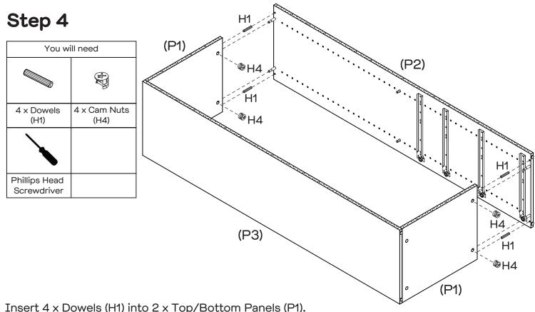
Insert 4 x Dowels (H1) into 2 x Top/Bottom Panels (P1).
