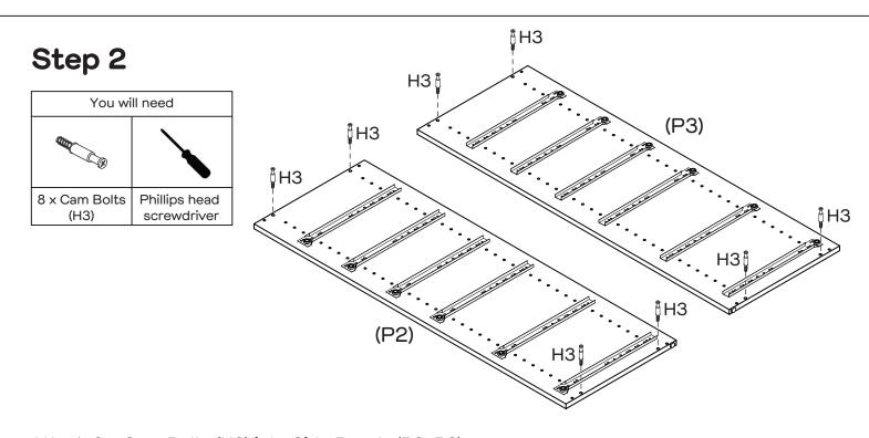
Attach 8 x Cam Bolts (H3) into Side Panels (P2, P3).
