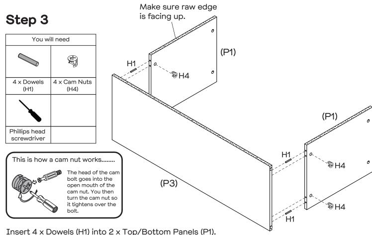
Insert 4 x Dowels (HI) into 2 x Top/Bottom Panels (PI).
