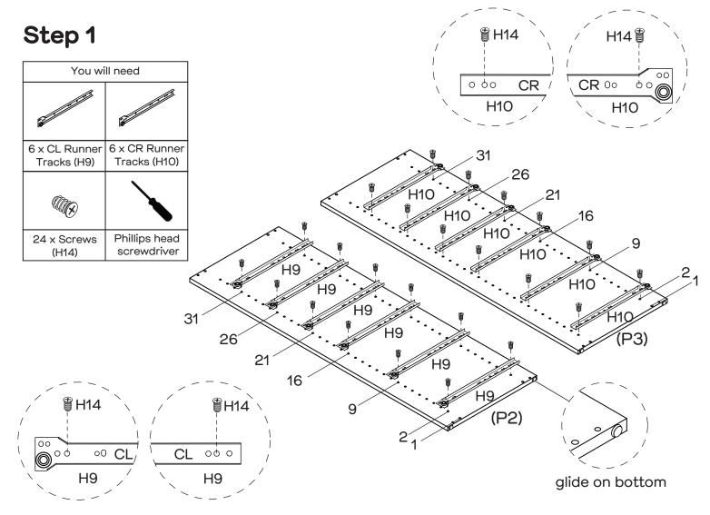
Attach 6 x CL Runner Tracks (H9) to Left Side Panel (P2) with 12 x Screws (H14). Attach 6 x CR Runner Tracks (H10) to Right Side Panel (P3) with 12 x Screws (H14).
