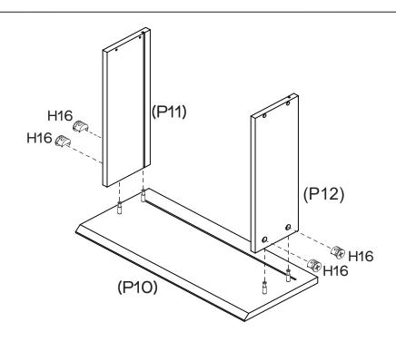
Insert 4 x Small Cam Nuts (H16) into the holes of Drawer Sides (P11, P12). Rotate the cam nuts so the arrows point towards the incoming cam bolts. Push Drawer Sides (P11, P12) into place and tighten the cam nuts.
