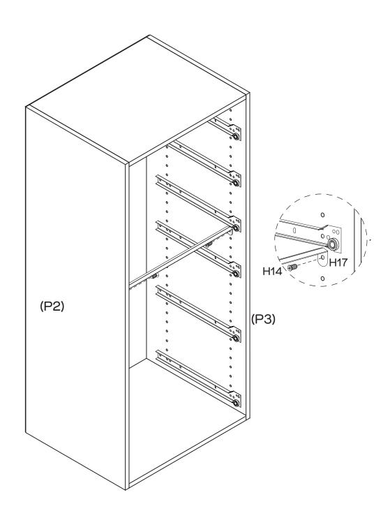
Attach Metal Bracket (H17) to Side Panels (P2, P3) with 2 x Screws (H14).
