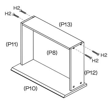
Attach Drawer Back (P13) to Drawer Sides (P11, P12) with 4 x Long Screws (H2), make sure that the groove lines up the whole way around the drawer.
