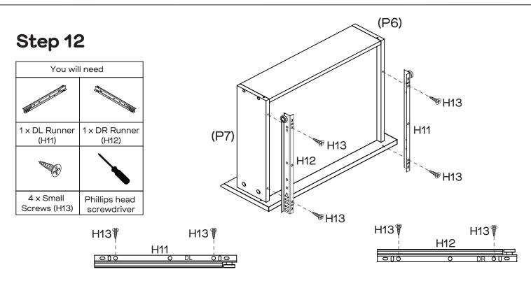
Attach 1 x DL Runner (H11) to the bottom of Small Left Drawer Side (P6) and 1 x DR Runner (H12) to the bottom of Small Right Drawer Side (P7) with 4 x Small Screws (H13).
