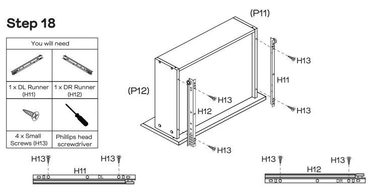
Attach 1 x DL Runner (H11) to the bottom of Left Drawer Side (P11) and 1 x DR Runner (H12) to the bottom of Right Drawer Side (P12) with 4 x Small Screws (H13).
