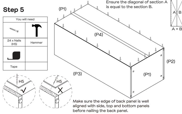
Attach Back Panel (P4) to the cabinet with  $24 \times \text{Nails}$  (H5) using hammer. Please measure with a tape to ensure that the spacing of the nails is consistent, and make sure the tip of the nails are vertically centered on the edge of the Side Panels(P2, P3) and Top/Bottom Panels (P1).
