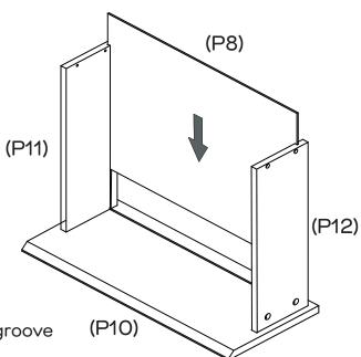
Slide Drawer Base (P8) into the groove in Drawer Sides (P11, P12).
