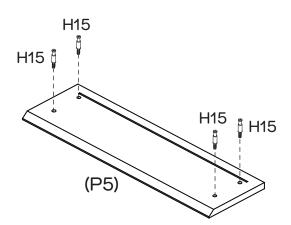
Attach 4 x Small Cam Bolts (H15) into Small Drawer Front (P5).
