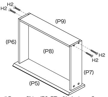
Attach Small Drawer Back (P9) to Small Drawer Sides (P6, P7) with 4 x Long Screws (H2), make sure that the groove lines up the whole way around the drawer.
