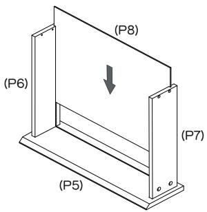
Slide Drawer Base (P8) into the groove in Small Drawer Sides (P6, P7).
