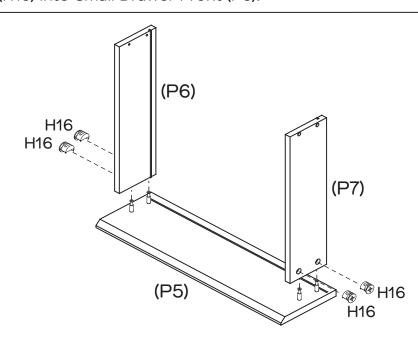
Insert 4 x Small Cam Nuts (H16) into the holes of Small Drawer Sides (P6, P7). Rotate the cam nuts so the arrows point towards the incoming cam bolts. Push Small Drawer Sides (P6, P7) into place and tighten the cam nuts.
