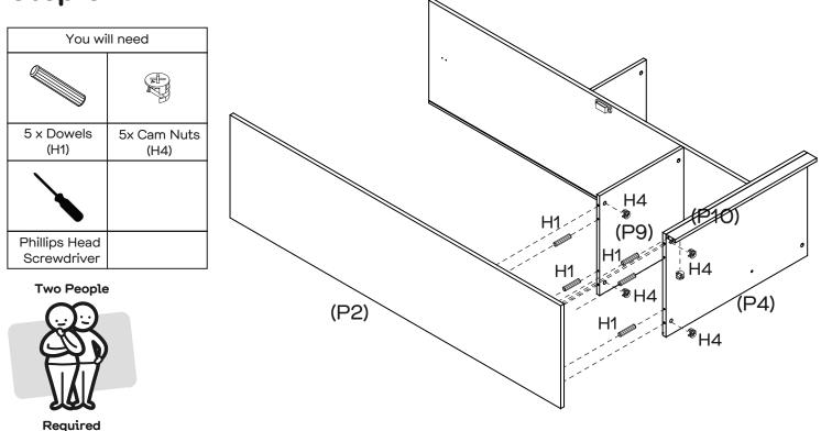
Insert 5 x Dowels (H1) into Shelf Panel (P9), Bottom Panel (P4) and Rail (P10). Insert 5 x Cam Nuts (H4) into Shelf Panel (P9), Bottom Panel (P4) and Rail (P10). Rotate the nuts so the arrows point towards the incoming bolts. Attach Left Side Panel (P2) to Shelf Panel (P9), Bottom Panel (P4) and Rail (P10) by tightening all nuts with the Phillips Head Screwdriver.
