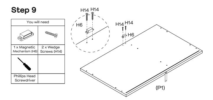
Attach 1  $\times$  Magnetic Mechanism (H6) to Top Panel (P1) with 2  $\times$  Wedge Screws (H14) as shown by tightening with the Phillips Head Screwdriver.
