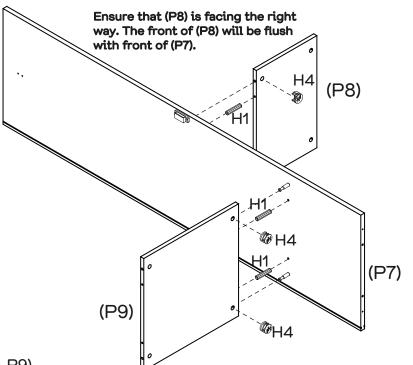
Insert 4 x Dowels (H1) into Shelf Panels (P8 & P9). Insert 4 x Cam Nuts (H4) into Shelf Panels (P8 & P9). Rotate the nuts so the arrows point towards the incoming bolts. Attach Shelf Panels (P8 & P9) to Divider (P7) by tightening all nuts with the Phillips Head Screwdriver.
