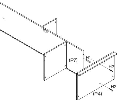
Insert 2 x Dowels (H1) into Divider (P7). Attach Bottom Panel (P4) to Divider (P7) with 2 x Long Screws (H2) by tightening with the Phillips Head Screwdriver.
