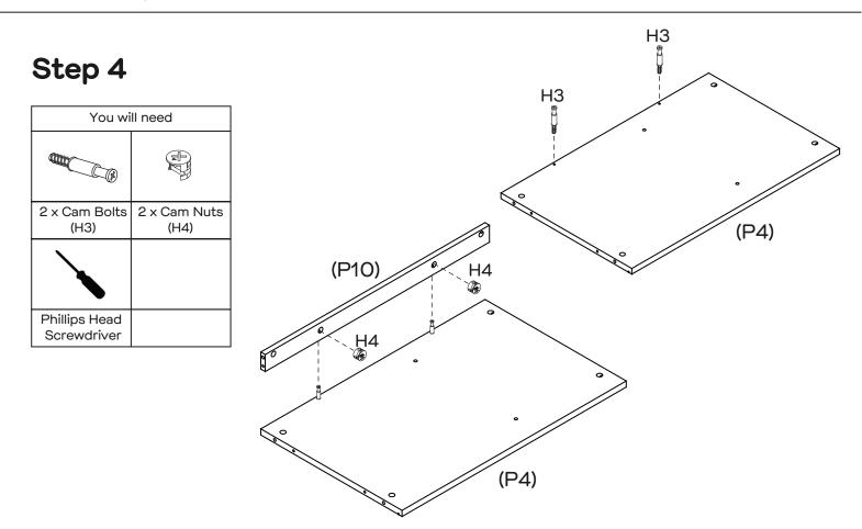
Insert 2 x Cam Bolts (H3) into Bottom Panel (P4). Tightening with the Phillips Head Screwdriver. Insert 2 x Cam Nuts (H4) into Rail (P10). Rotate the nuts so the arrows point towards the incoming bolts. Attach Rail (P10) to Bottom Panel (P4) by tightening all nuts with the Phillips Head Screwdriver.
