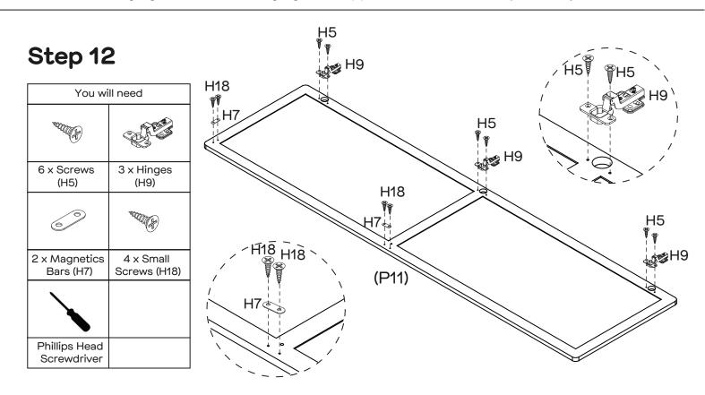
Attach 2 x Magnetics Bars (H7) to Door (P11) with 4 x Small Screws (H18). Attach 3 x Hinges (H9) to Door (P11) with 6 x Screws (H5). Tightening with the Phillips Head Screwdriver.
