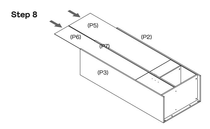
Slide Back Panels (P5 & P6) into the grooves of Left & Right Side Panel (P2 & P3) and Divider (P7).
