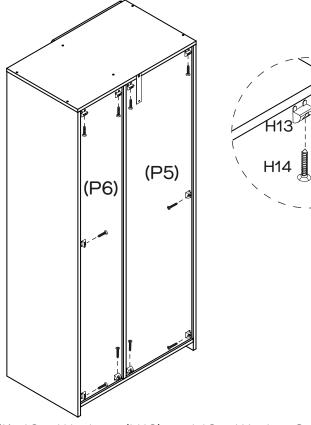
Secure Back Panels (P5 & P6) in place with 10  $\times$  Wedges (H13) and 10  $\times$  Wedge Screws (H14) by tightening with the Phillips Head Screwdriver.
