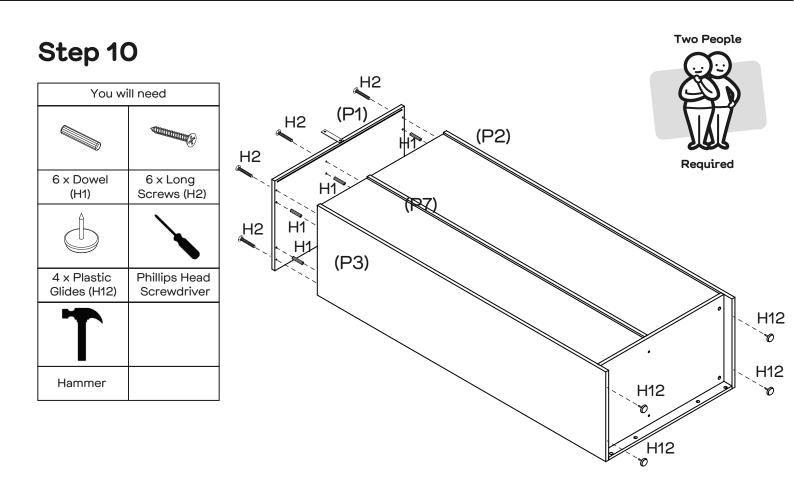
Insert 6 x Dowels (H1) into Left & Right Side Panel (P2 & P3) and Divider (P7). Attach Top panel (P1) to Left & Right Side Panel (P2 & P3) and Divider (P7) with 6 x Long Screws (H2) by tightening with the Phillips Head Screwdriver.
