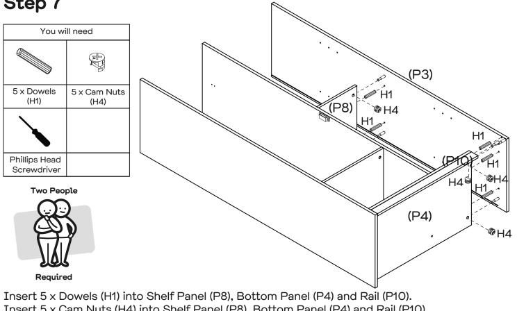
Insert 5 x Cam Nuts (H4) into Shelf Panel (P8), Bottom Panel (P4) and Rail (P10). Rotate the nuts so the arrows point towards the incoming bolts. Attach Right Side Panel (P3) to Shelf Panel (P8), Bottom Panel (P4) and Rail (P10) by tightening all nuts with the Phillips Head Screwdriver.
