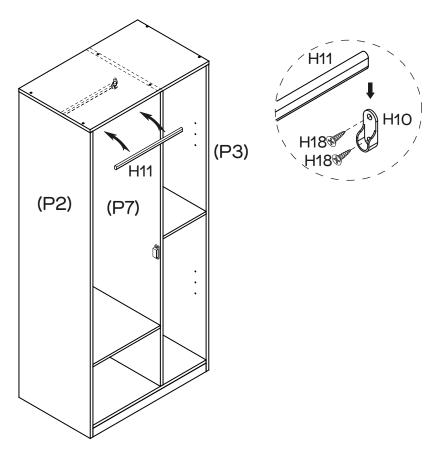
Attach 2 x Hanging Rail Supports (H10) to the Left Side Panels (P2) and Divider (P7) with 4 x Small Screws (H18) by tightening with a Phillips Head Screwdriver. Attach 1 x Hanging Rail (H11) to Hanging Rail Support (H10) as shown by slotting it in.
