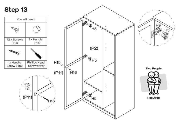
Attach Door (P11) to Left Side Panel (P2) with 12 x Screws (H5). Attach 1 x Handle (H15) to Door (P11) with 1 x Handle Screw (H16). Tightening with the Phillips Head Screwdriver.
