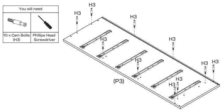
Attach 10 x Cam Bolts (H3) to Left Side Panel (P3) as shown by tightening with the Phillips Head Screwdriver.
