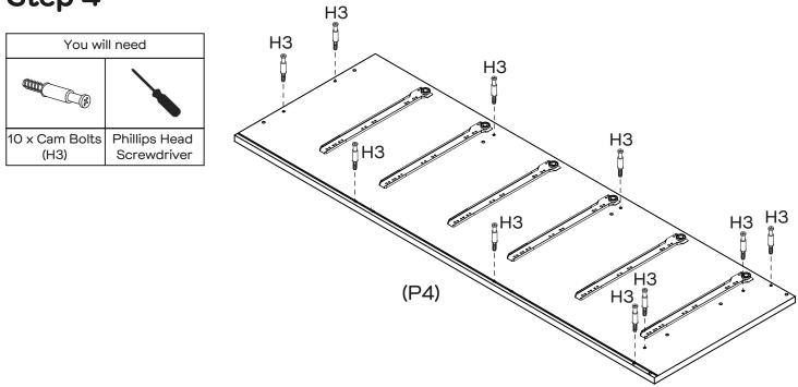
Attach 10 x Cam Bolts (H3) to Right Side Panel (P4) as shown by tightening with the Phillips Head Screwdriver.
