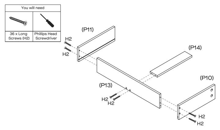
Attach Drawer Back (P13) to Left & Right Drawer Sides (P10 & P11) and Rail (P14) with 6 x Long Screws (H2) by tightening with the Phillips Head Screwdriver. Repeat this step for the remaining Drawer Backs (P13 x 5), Drawer Sides (P10 x 5 & P11 x 5) and Rails (P14 x 5).
