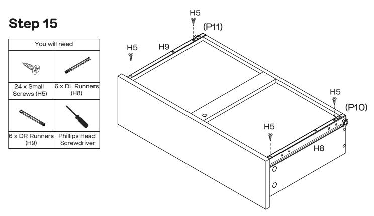
Attach 1 x DL Runner (H8) to the bottom of Left Drawer Side (P10) and 1 x DR Runner (H9) to the bottom of Right Drawer Side (P11) with 4 x Small Screws (H5) by tightening with the Phillips Head Screwdriver. Repeat this step for the remaining five Drawers.
