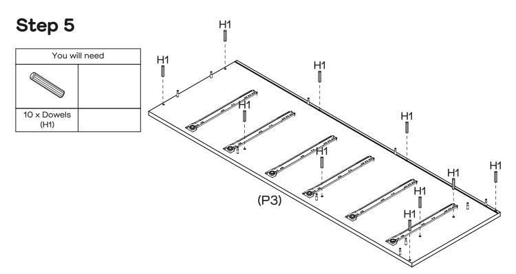
Insert 10 x Dowels (H1) into Left Side Panel (P3) as shown.
