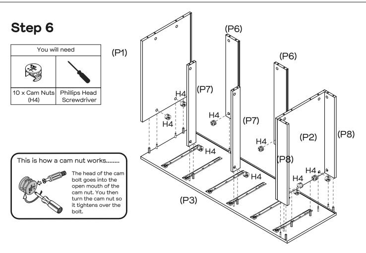
Insert 10 x Cam Nuts (H4) into Top Panel (P1), Base Panel (P2) and Rails (P6 x 2, P7 x 2, P8 x 2). Rotate the nuts so the arrows point towards the incoming bolts. Attach Top Panel (P1), Base Panel (P2) and Rails (P6 x 2, P7 x 2, P8 x 2) to Left Side Panel (P3) by tightening all nuts with the Phillips Head Screwdriver.
