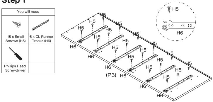
Attach  $6 \times CL$  Runner Tracks (H6) to Left Side Panel (P3) with  $18 \times Small Screws$  (H5) by tightening with the Phillips Head Screwdriver.
