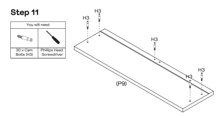
Attach 5 x Cam Bolts (H3) to Drawer Front (P9) as shown by tightening with the Phillips Head Screwdriver. Repeat this step for the remaining five Drawer Fronts (P9 x 5).
