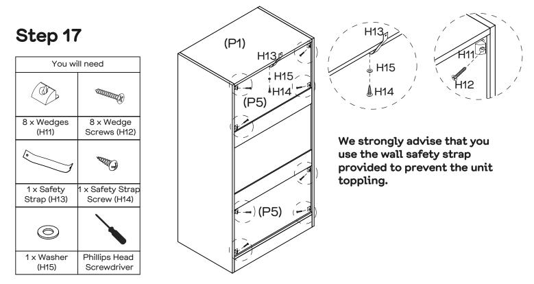
Secure Back Panels (P5 x 2) in place with 8 x Wedges (H11) and 8 x Wedge Screws (H12) by tightening with the Phillips Head Screwdriver. Attach the Safety Strap (H13) to the Top Panel (P1) with 1 x Safety Strap Screw (H14) & 1 x Washer (H15) by tightening with the Phillips Head Screwdriver.
