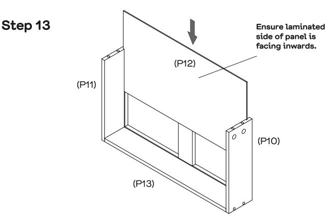
Slide Drawer Base (P12) into the grooves of Left & Right Drawer Sides (P10 & P11) and Drawer Back (P13). Repeat this step for the remaining Drawer Bases (P12 x 5).
