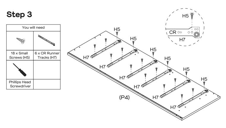
Attach 6 x CR Runner Tracks (H7) to Right Side Panel (P4) with 18 x Small Screws (H5) by tightening with the Phillips Head Screwdriver.
