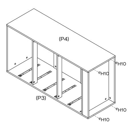
Secure 4 x Plastic Glides (H10) to the bottom of Left & Right Side Panels (P3 & P4) as shown using the Hammer.
