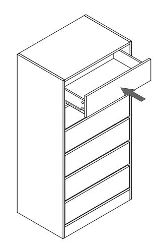
Gently insert the assembled drawers into the unit by carefully lining up the drawer runners with the drawer runner tracks.
