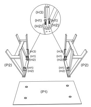
Align the Trestle Leg (P2) screw holes with the metal plates on the Glass Top (P1). Use 4 x Washers (H2) and 4 x Bolts (H1) to secure the Trestle Leg (P2) to the Glass Top (P1) by tightening with the Allen Key (H3). Repeat steps to attach the second Trestle Leg (P2).
