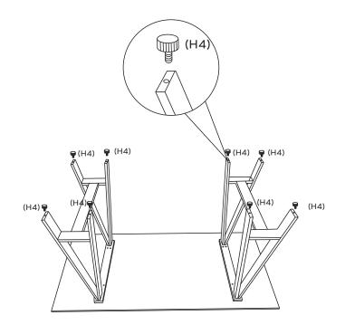
Screw in 8 x Levelling Feet (H4) to the bottom of Trestle Legs (P2x2). If your floor is uneven the levelling feet can be adjusted to make the desktop level.
