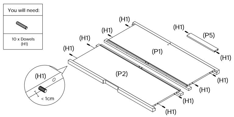
Insert 10 x Dowels (H1) into Back Panel (P1), Front Panel (P2) and Support Bar (P5) as shown.
