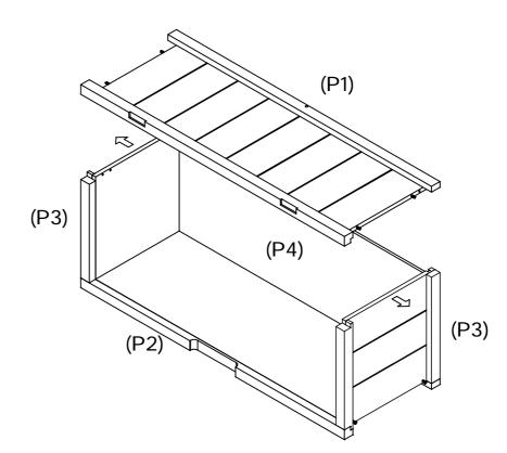
Attach Back Panel (P1) to Side Panels (P3x2) and Support Bar (P5) as shown by gently slotting the dowels into place. Ensure all dowels are attached and the Bottom Panel (P4) is slotted in the grooves of all panels correctly.
