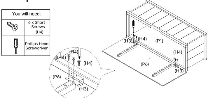
Secure Top Panel (P6) to 2 x Hinges (H3) as shown with 6 x Short Screws (H4) by tightening with the Phillips Head Screwdriver.
