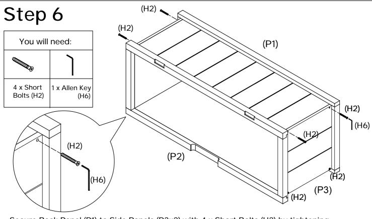
Secure Back Panel (P1) to Side Panels (P3x2) with 4 x Short Bolts (H2) by tightening with the Allen Key (H6). Finally, tightening the remaining 4 x Short Bolts (H2) to 100%.
