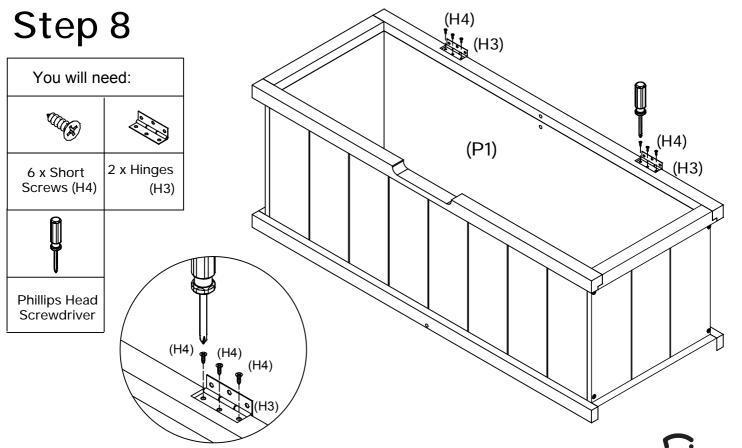
Attach 2 x Hinges (H3) to Back Panel (P1) as shown with 6 x Short Screws (H4) by tightening with the Phillips Head Screwdriver.
