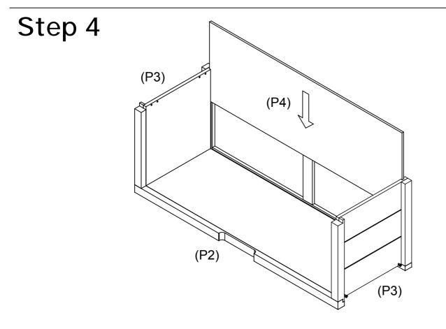
Insert Bottom Panel (P4) into the grooves of Front Panel (P2) and Side Panels (P3x2).
