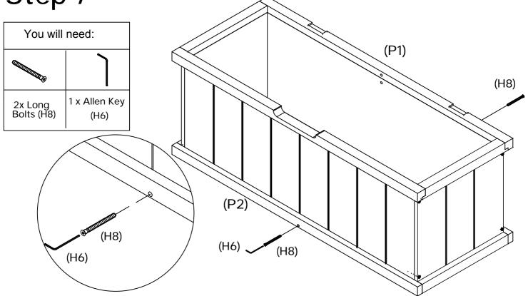
Secure Support Bar (P5) to Back & Front Panels (P1&P2) with 2 x Long Bolts (H8) by tightening with the Allen Key (H6).
