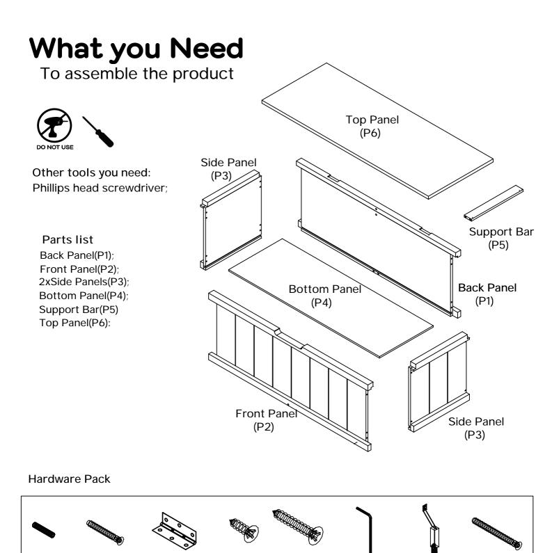
10 x Dowels8 x Short2 x Hinges14 x Short2 x Long1 x Allen Key1 x Support(H1)Bolts(H3)ScrewsScrews(H6)Hinge(H2)(H4)(H5)(H7)
