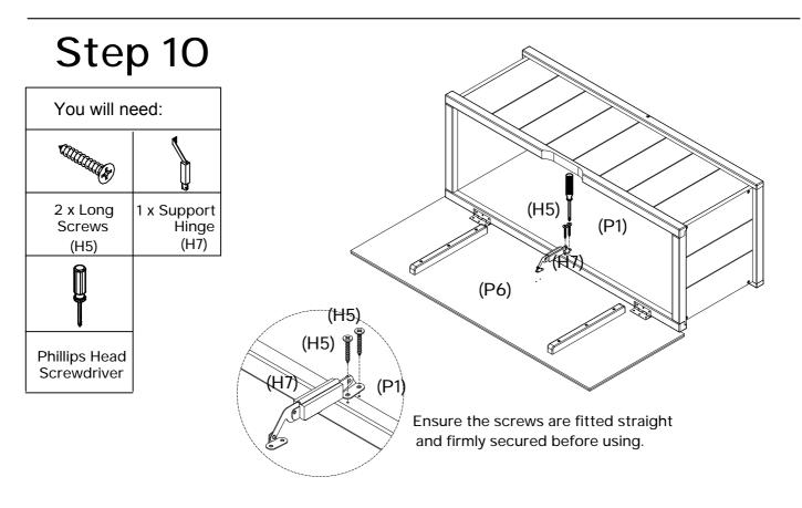
Attach Support Hinge (H7) to Back Panel (P1) as shown with 2 x Long Screws (H5) by tightening with the Phillips Head Screwdriver .
