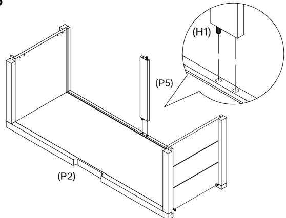
Attach Support Bar (P5) to Front Panel (P2) as shown. Ensure the dowel is placed into the correct hole.
