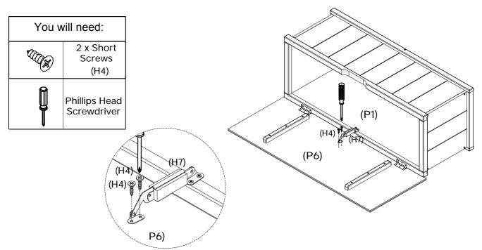
Attach Support Hinge (H7) to Top Panel (P6) as shown with 2 x Short Screws (H5) by tightening with the Phillips Head Screwdriver.
