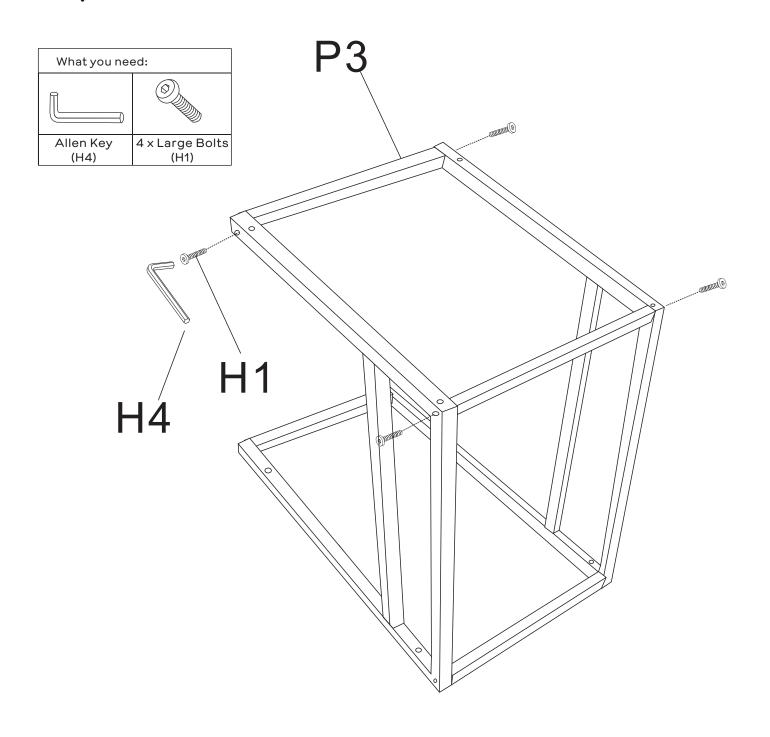
Align 2 x support bars (P3) between the 2 x table leg frames (P2). Attach using 4 x Large Bolts (H1) tightening with the allen key (H4). You may now fully tighten all bolts securing the support bars (P3) to the table leg frames (P2).
