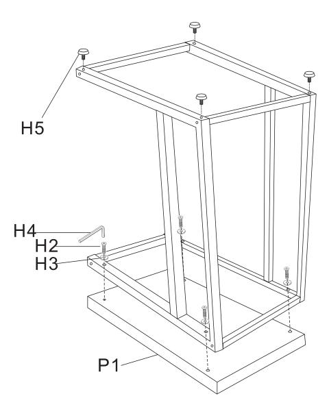
Place the assembled frame (P2,P3) onto Table Top (P1). Align the holes on the Leg Frames (P2) with the holes on the Table Top (P1).
