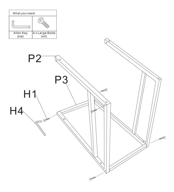
Align 2 x Support Bars (P3) between the 2 x Table Leg Frame (P2). Attach using 4 x Large Bolts (H1) tightening with the Allen Key (H4). Do not fully tighten the bolts until Step 2.
