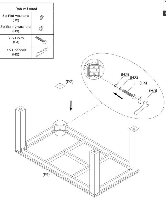
Put spring washer (H3) and then flat washer (H2) onto bolt (H4). Align the legs (P2) with table top (P1) and fix with bolt (H4). Use spanner (H5) to tighten.
