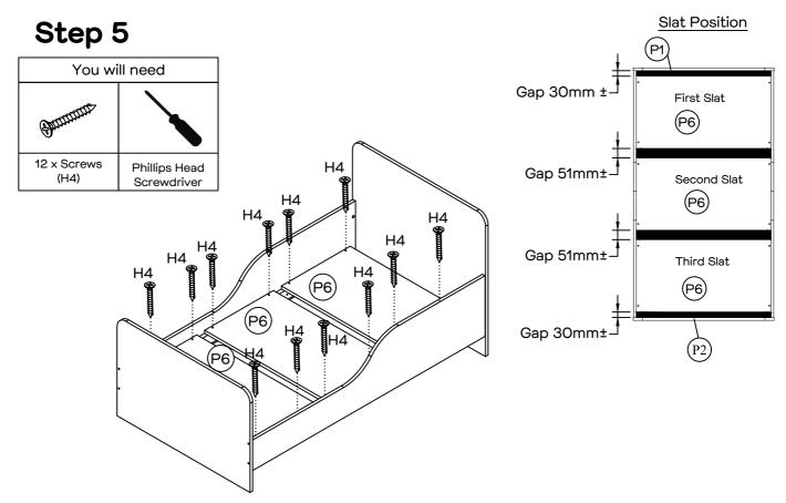
Secure panels (P6) with 12 x screws by using a philips head screwdriver. Please note the gap dimensions in the above diagram.
