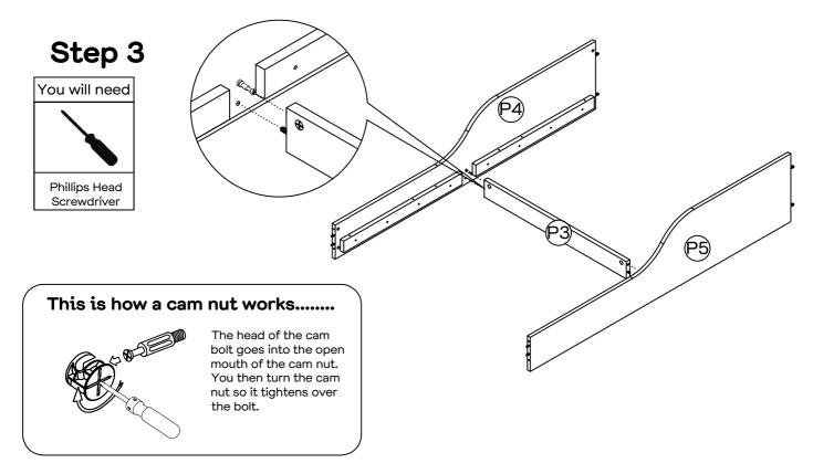
Attach panels (P4) & (P5) to panel (P3). Turn the cam nuts on panel (P3) clockwise with a phillips head screwdriver to lock in position.
