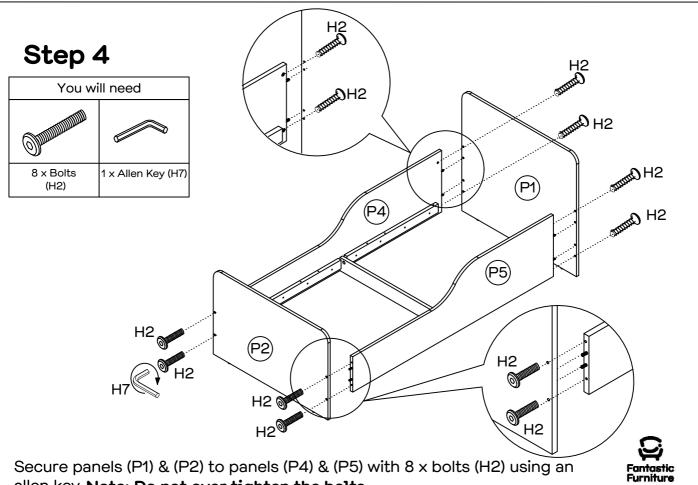
allen key. Note: Do not over tighten the bolts.
