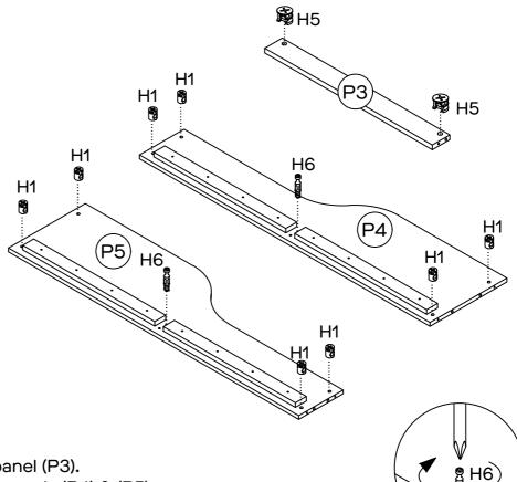
Insert 2 x cam nuts (H5) into panel (P3).
