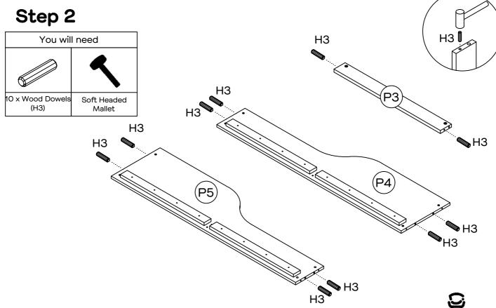
Insert 10 x dowels (H3) into panels (P3), (P4) & (P5) by hand or gently using a soft headed mallet.
