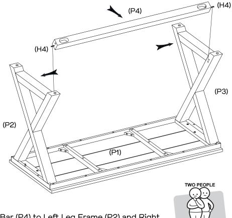
Attach Cross Bar (P4) to Left Leg Frame (P2) and Right Leg Frame (P3) as shown.
