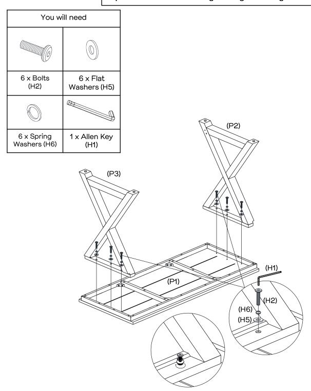
Lay the Table Top (P1) upside down, attach Left Leg Frame (P2) with  $3 \times 9$  Spring Washers (H6)  $3 \times 9$  Flat Washers (H5),  $3 \times 9$  Bolts (H2), using the Allen Key (H1). Only Tighten  $3 \times 9$  Bolts (H2) to 80%.
