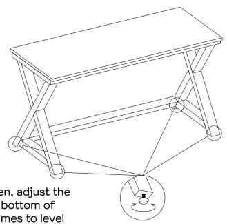
If your floor is uneven, adjust the levelling feet on the bottom of Right & Left Leg Frames to level the desktop.
