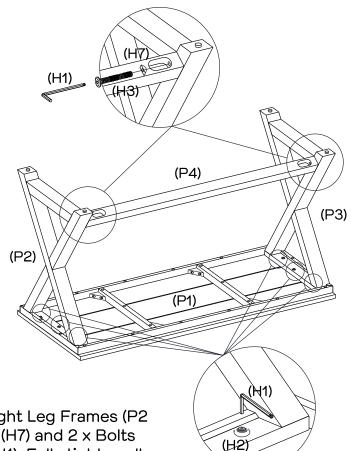
Secure Cross Bar (P4) to Left & Right Leg Frames (P2 & P3) with 2 x Half Moon Washers (H7) and 2 x Bolts (H3) by tightening with Allen Key (H1). Fully tighten all Bolts as shown.
