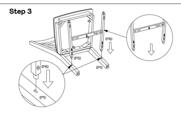
Attach Left Cross Bar (P5), Cross Bar (P7) and Right Cross Bar (P6) into Backrest (P1) as shown.
