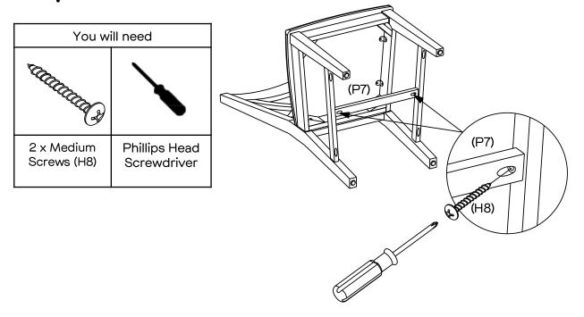
Attach 2 x Medium Screws (H8) into Cross Bar (P7) using a Phillips head screwdriver.
