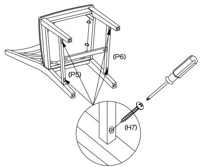
Attach  $4 \times \text{Large Screws}$  (H7) into Left Cross Bar (P5) and Right Cross Bar (P6) using a Phillips head screwdriver.
