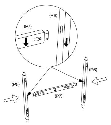
Attach Left Cross Bar (P5) , Cross Bar (P7) and Right Cross Bar (P6) as shown above.
