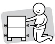
Unless instructed, do not fully tighten screws until the item is full assembled.
