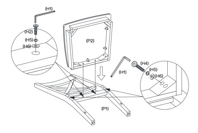
Attach the Seat Box (P2) to Backrest (P1) with 2  $\times$  Small Bolts (H2) and 4  $\times$  Large Bolts (H4), 6  $\times$  Spring Washers (H5) and 6  $\times$  Flat Washers (H6), tightening with Allen Key (H1). Do not fully tighten the Bolts until Step 7.
