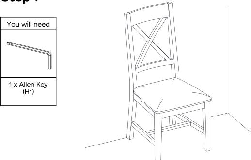
Carefully turn chair to its upright position. Ensure chair is leveled to the ground. Adjust leg balance if needed.
