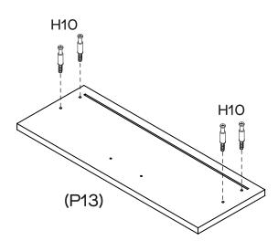
Secure 4 x Small Cam Bolts (H10) to Drawer Fronts (P13) by tightening with the Phillips Head Screwdriver.
