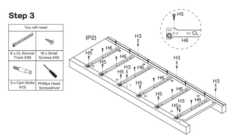
Attach  $6 \times CL$  Runner Tracks (H6) to Left Side Panel (P2) with  $18 \times Small$  Screws (H5). Secure  $5 \times Cam$  Bolts (H3) to Left Side Panel (P2) by tightening with the Phillips Head Screwdriver.
