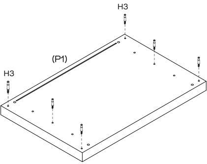
Secure 6 x Cam Bolts (H3) to Top Panel (P1) by tightening with the Phillips Head Screwdriver.
