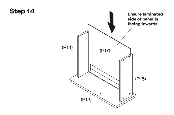
Slide the Drawer Base (P17) into the grooves of Left & Right Drawer Sides (P14 & P15) as shown.
