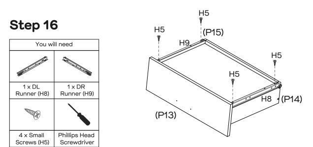
Attach 1  $\times$  DL Runner (H8) to Left Drawer Side (P14) and 1  $\times$  DR Runner (H9) to Right Drawer Side (P15) with 4  $\times$  Small Screws (H5) by tightening with the Phillips Head Screwdriver.
