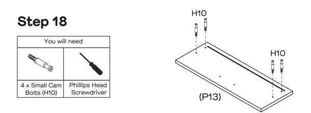
Secure 4 x Small Cam Bolts (H10) to Drawer Fronts (P13) by tightening with the Phillips Head Screwdriver.
