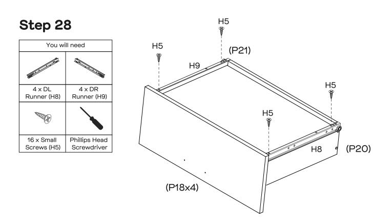
Attach 4 x DL Runner (H8) to Left Drawer Side (P20x4) and 4 x DR Runner (H9) to Right Drawer Side (P21x4) with 16 x Small Screws (H5) by tightening with the Phillips Head Screwdriver.
