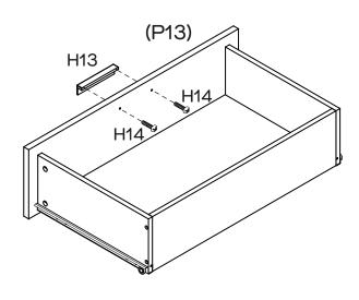
Attach 1  $\times$  Handles (H13) to Drawer Fronts (P13) with 2  $\times$  Handle Bolts (H14). Tighten Round Head Bolts using a Phillips head screwdriver.
