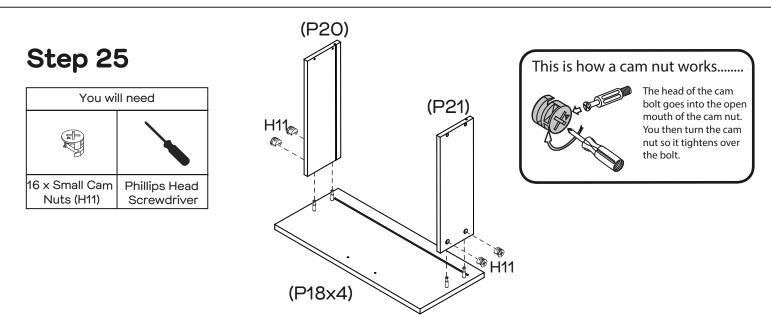
Insert 16 x Small Cam Nuts (H11) into Left & Right Drawer Sides (P20x4 & P21x4), attach to Drawer Fronts (P18x4) by tightening Cam Nuts with the Phillips Head Screwdriver.
