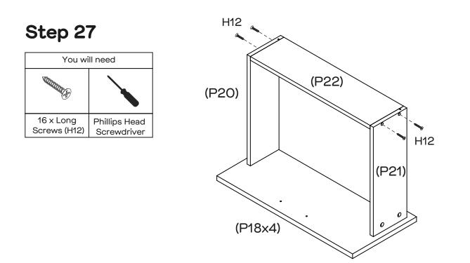
Attach Drawer Back (P22x4) to Left & Right Drawer Sides (P20x4 & P21x4) with 16 x Long Screws (H12) by tightening with the Phillips Head Screwdriver. Before securing - Ensure the Bottom Panel lines up with the grooves the whole way around the drawer.
