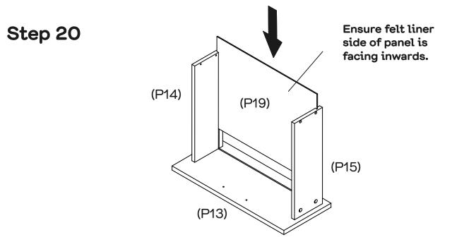
Slide the Felt Drawer Base (P19) with the felt liner into the grooves of Left & Right Drawer Side (P14 & P15) as shown.
