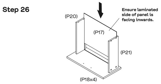
Slide the Drawer Bases (P17x4) into the grooves of Left & Right Drawer Side (P20x4 & P21x4) as shown.
