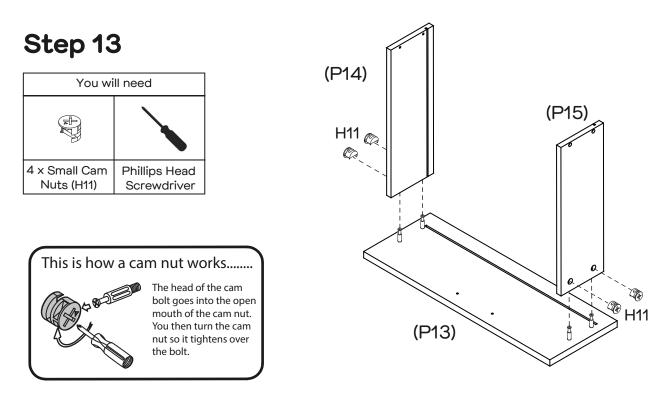
Insert 4 x Small Cam Nuts (H11) into Left & Right Drawer Sides (P14 & P15), attach to Drawer Fronts (P13) by tightening Cam Nuts with the Phillips Head Screwdriver.
