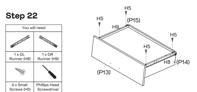
Attach 1 x DL Runner (H8) to Left Drawer Side (P14) and 1 x DR Runner (H9) to Right Drawer Side (P15) with 4 x Small Screws (H5) by tightening with the Phillips Head Screwdriver.
