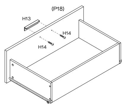
Attach 4 x Handles (H13) to Drawer Front (P18x4) with 8 x Handle Bolts (H14). Tighten Round Head Bolts using a Phillips head screwdriver.
