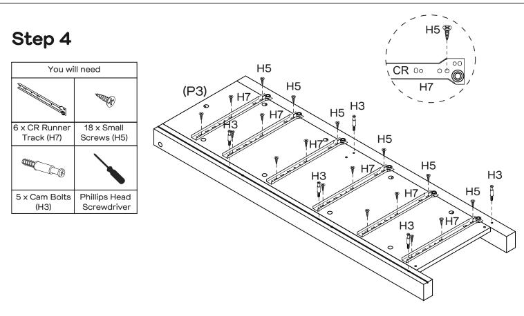
Attach 6 x CR Runner Tracks (H7) to Right Side Panel (P3) with 18 x Small Screws (H5). Secure 5 x Cam Bolts (H3) to Right Side Panel (P3) by tightening with the Phillips Head Screwdriver.
