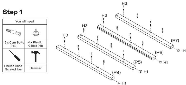
Secure 16 x Cam Bolts (H3) to Legs(P4, P5, P6, P7) by tightening with the Phillips Head Screwdriver. Hammer 4 x Plastic Glides (H1) on Legs (P4, P5, P6, P7) as shown.
