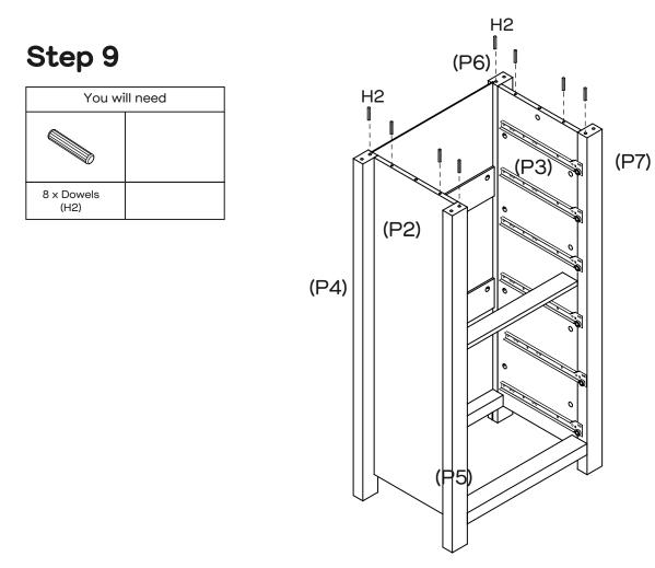
Insert 8 xDowels (H2) into Left Side Panel (P2), Right Side Panel (P3) and Legs (P4, P5, P6, P7).
