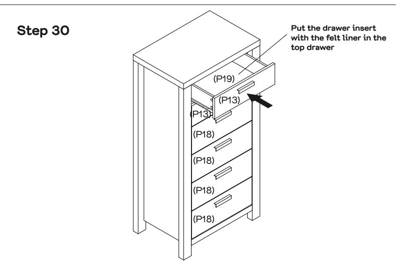
Insert the assembled drawer into the unit by gently guiding the drawer runners into place.
