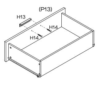
Attach 1 x Handles (H13) to Drawer Front (P13) with 2 x Handle Bolts (H14). Tighten Round Head Bolts using a Phillips head screwdriver.
