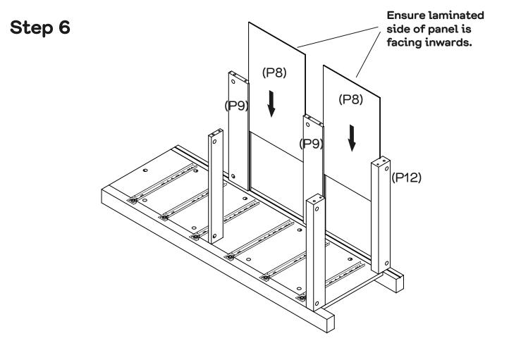
Slide 2 x Back Panels (P8) into the grooves of Rails (P9x2&P12).
