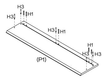
Insert 5 x Dowels (H1) into Drawer Front (P1). Attach 5 x Small Cam Bolts (H3) to Drawer Front (P1).
