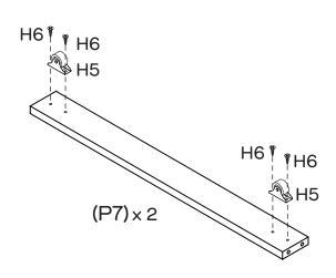
Attach 2 x Wheels (H5) to Drawer Support (P7) with 4 x Small Screws (H6). Repeat Step 2 again with the other Drawer Support (P7).
