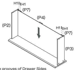
Slide Drawer Base (P4) in through the grooves of Drawer Sides (P2, P3). Insert  $4 \times 1$  Dowels (H1) into Drawer Supports (P7).
