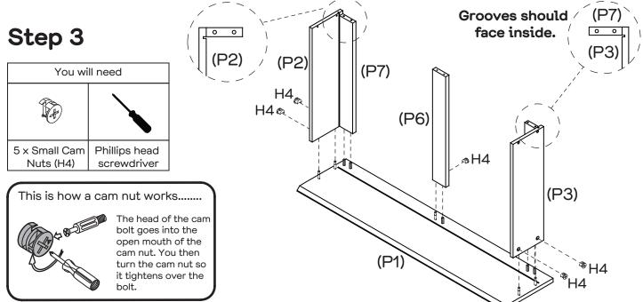
Insert 5 x Small Cam Nuts (H4) into the holes of Drawer Sides (P2, P3) and Central Drawer Support (P6). Rotate the cam nuts so the arrows point towards the incoming cam bolts. Align and secure Drawer Sides (P2, P3) and Drawer Supports (P6, P7) into place, and then tighten the cam nuts.
