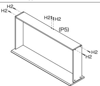
Attach Drawer Back (P5) to Drawer Sides (P2, P3) and Central Drawer Support (P6) with 6 x Long Screws (H2). Make sure that the groove lines up the whole way around the drawer. Repeat Step 1 to Step 5 to assemble the other drawer.
