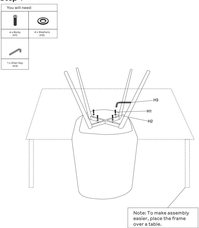
Align holes on seat (P1) with holes on metal frame (P2). Attach seat (P1) to metal frame (P2) using 4 x bolts (H1) and 4 x washers (H2). Apply downward pressure on the metal frame (P2) to secure the bolts (H1) into the pre-drilled holes and hand-tighten by turning the bolts (H1) clockwise. Once the bolts (H1) are secure, use the allen key (H3) to firmly tighten the bolts (H1).
