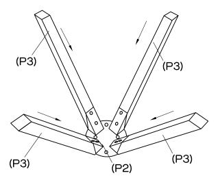
Position the  $4 \times legs$  (P3) onto the base (P2) as shown.
