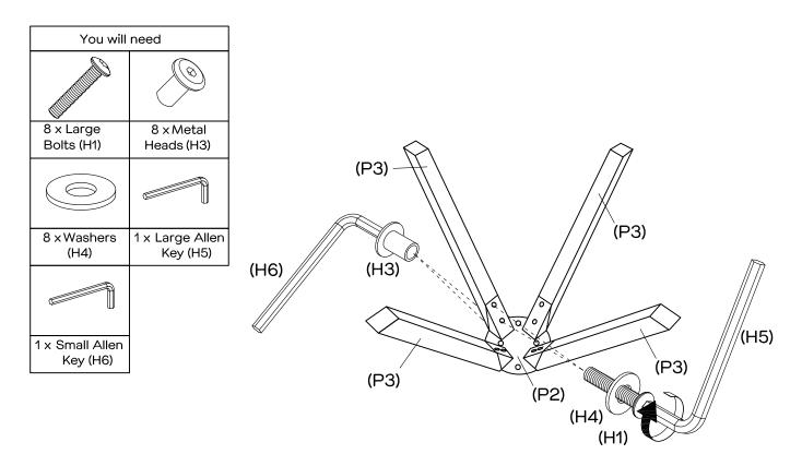
Attach the 1 x leg (P3) to the base (P2) using 2 x metal heads (H3), 2 x washers (H4) and 2 x large bolts (H1), completely tightening using the large allen key (H5) and small allen key (H6) as shown.
