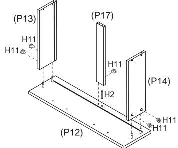
Insert 1 x Small Dowel (H2) into Drawer Front (P12) as shown.
