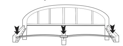
Insert the full slat into the side rail and centre rail one by one.
