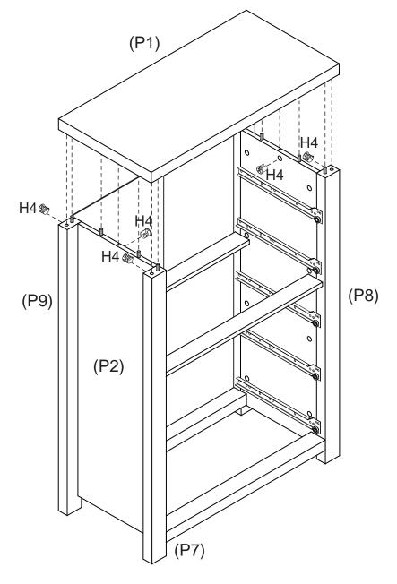
Insert 6 x Cam Nuts (H4) into the holes of Side Panels (P2, P3) and Legs (P7, P8, P9, P10). Rotate the cam nuts so the arrows point towards the incoming cam bolts. Attach Top Panel (P1) into place, and then tighten the cam nuts.
