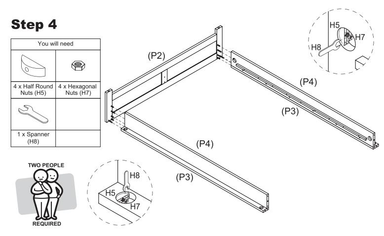
Attach Bedfoot (P2) to Side Covers (P3) and Side Rails (P4) with 4 x Half Round Nuts (H5) and 4 x Hexagonal Nuts (H7) using Spanner (H8).
