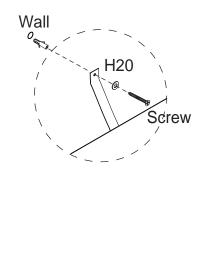
Move the tallboy to the final position, and attach the safety strap to the wall securely. Make sure it is firmly attached and snug fit.
