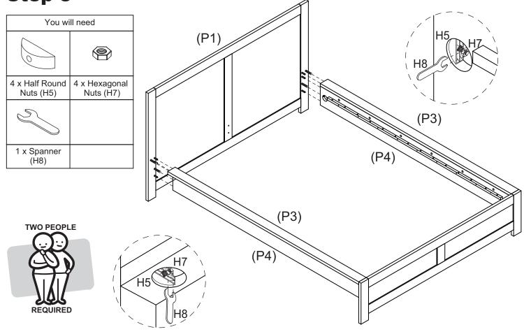
Attach Bedhead (P1) to Side Covers (P3) and Side Rails (P4) with 4 x Half Round Nuts (H5), and 4 x Hexagonal Nuts (H7) using Spanner (H8).
