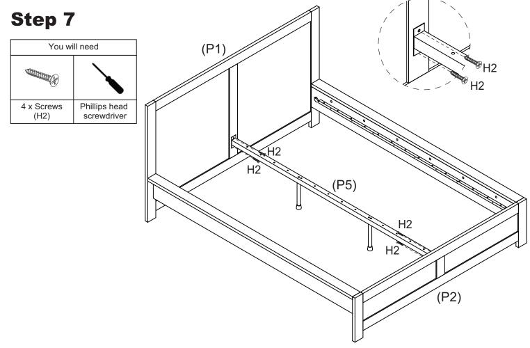
Attach Centre Rail (P5) to Bedhead (P1) and Bedfoot (P2) as shown. Then screw Centre Rail (P5) with 4 x Screws (H2).
