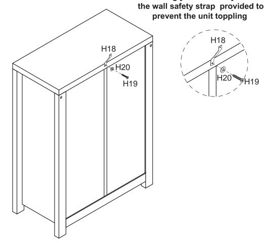
Use Screw (H19) and Washer (H20) to attach Safety Strap (H18) securely on Top Panel (P1) as shown. www.fantasticfurniture.com.au
