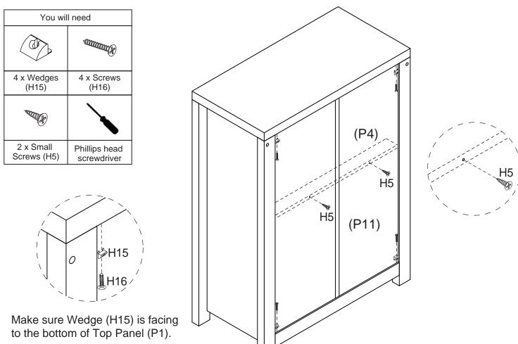
Secure Back Panel (P11) in place with 4 x Wedges (H15) using 4 x Screws (H16). Use 2 x Small Screws (H5) to fix Back Panel (P11) onto Rail (P4). Tighten the screws with a Phillips head screwdriver.
