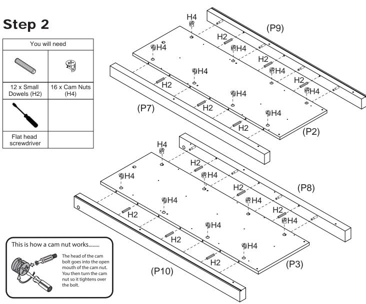
Insert 12 x Small Dowels (H2) into the holes of Side Panels (P2, P3).
