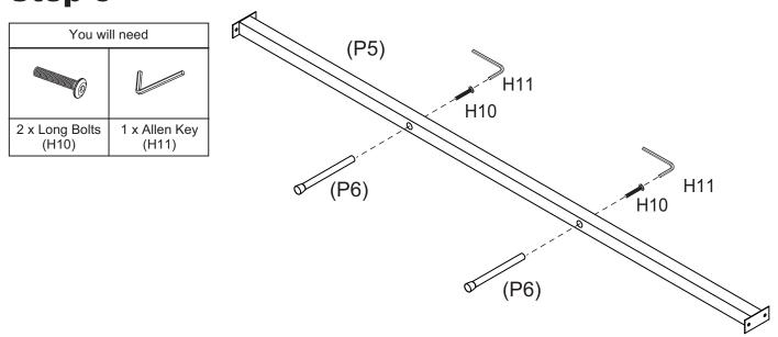
Attach 2 x Support Legs (P6) to Centre Rail (P5) with 2 x Long Bolts (H10) using Allen Key (H11).
