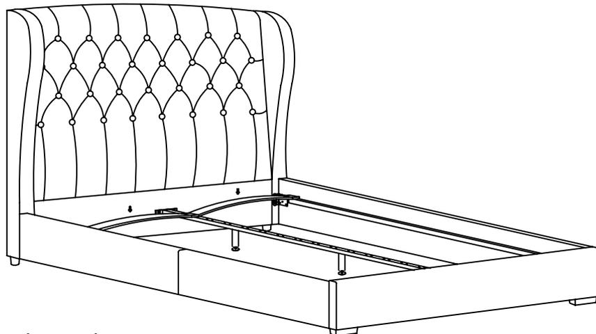
Sometimes it makes it easier to line up the hole if you press down in the middle of the slat to flatten it out.
