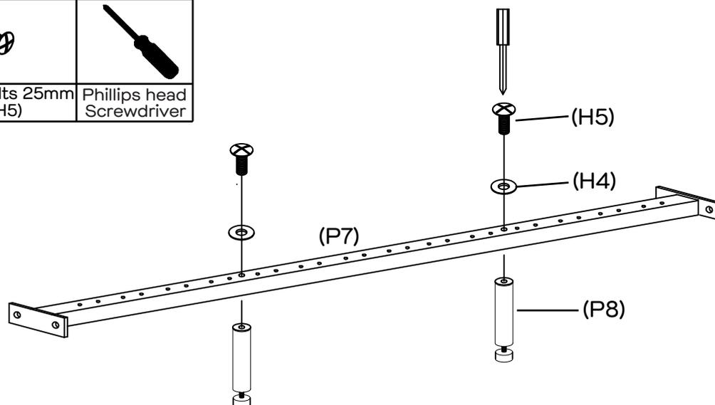
Attach 2 x support legs (P8) to the centre rail (P7) using 2 x Bolts (H5) and 2 x Washers (H4) as shown.
