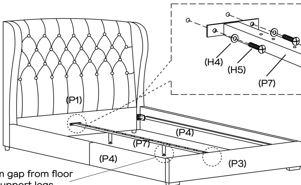
Adjust to be 10mm gap from floor to the bottom of support legs.
