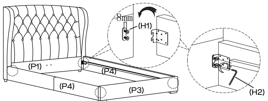
Install the bolts (H1) to the brackets by using Allen key (H2) as shown, do not tighten the bolts and keep them 8 mm loose. Then attach 2 x side rails (P4) to headboard (P1) and footboard (P3) by slotting the bracket on the side rails (P4) over the bolt as shown. No need to tighten bolts until step 8 .
