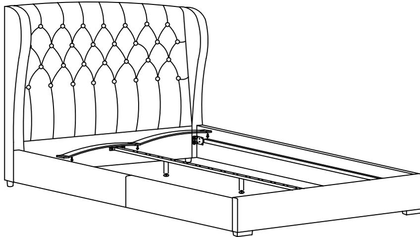
Insert the full slat into the side rail and centre rail one by one.
