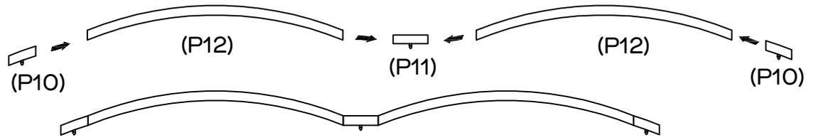
Push 2 End Connectors (P10), 2 pcs Slats (P12) and a Centre Connector (P11) together.
