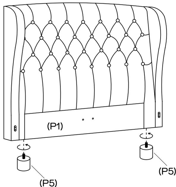
Attach 2 x headboard legs (P5) to the bottom of headboard (P1) as shown.
