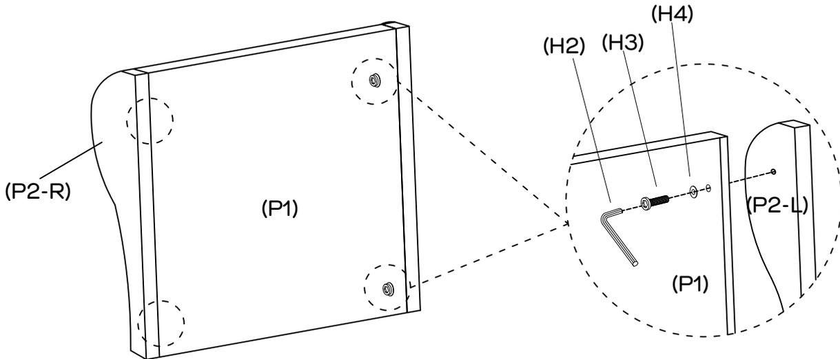
Attach wing (P2-L;P2-R) to the headboard (P1) with 4 x washers (H4) and 4 x bolt 45mm (H3) by using allen key (H2) as shown.
