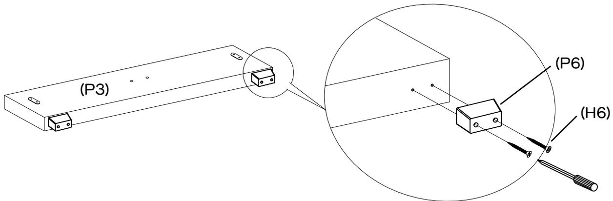
Attach 2 x footboard leg (P6) to the bottom of footboard (P3) with 4 x Large Screw 51mm (H6) by using phillips head screwdriver (not provided).
