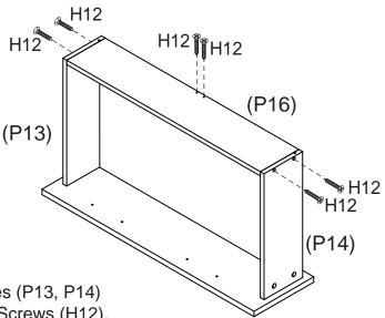
Attach Drawer Back (P16) to Drawer Sides (P13, P14) and Drawer Support (P17) with 6 x Long Screws (H12),
