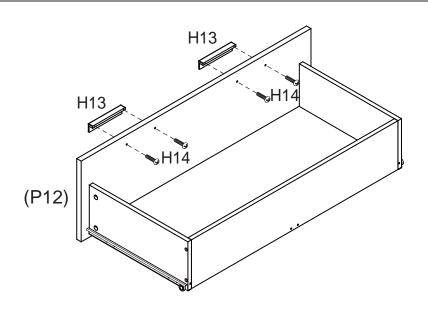
Attach 2 x Handles (H13) to Drawer Front (P12) with 4 x Round Head Bolts (H14). Tighten Round Head Bolts using a Phillips head screwdriver.
