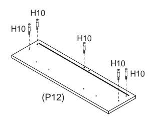
Screw 5 x Small Cam Bolts (H10) into Drawer Front (P12) with a Phillips head screwdriver.
