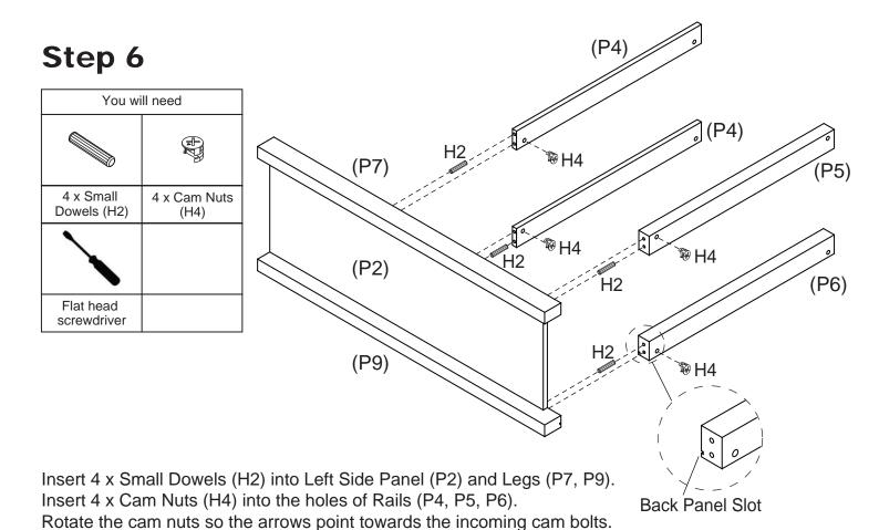
Attach Rails (P4, P5, P6) to the left frame, then tighten the cam nuts using a Flat head screwdriver.
