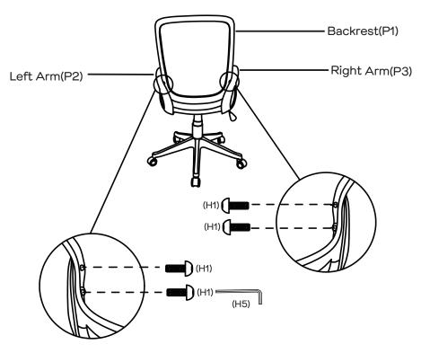
Slide the Backrest (P1) in between the Left & Right Arms (P2&P3) and align the bolt holes on each side. Secure the Backrest (P1) to Left & Right Arms (P2&P3)with 4x Short Bolts(H1)by tightening with the Allen Key(H5).
