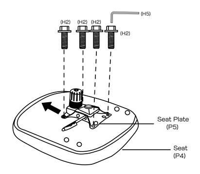
Note the front facing orientation of the Seat Plate (P5) and align the holes on the Seat Plate (P5) with the bottom of the Seat (P4) as shown. Secure the Seat Plate (P5) to the Seat(P4) with 4x Medium Bolts(H2) by tightening with the Allen Key(H5).
