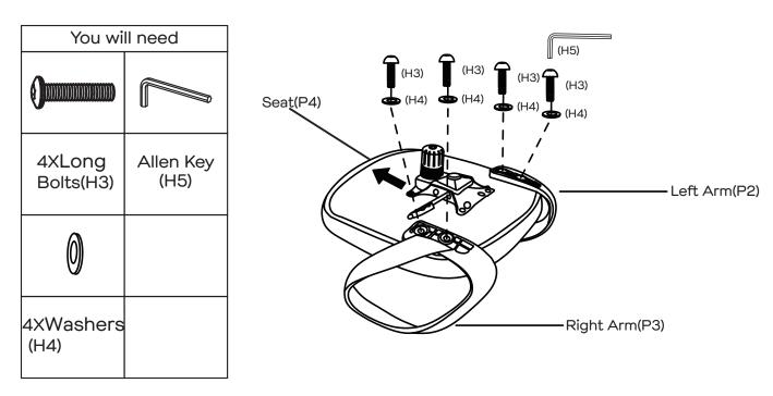
Attach Left & Right Arms (P2&P3) to Seat (P4) with 4 x Long Bolts (H3) and 4 x Washers (H4) as shown by tightening with the Allen Key (H5).
