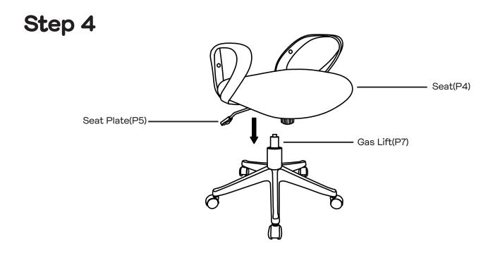
Position the centre hole of the Seat Plate(P5) over the top of Gas Lift(P7). Carefully lower the Seat(P4) onto the Gas Lift(P7). Press seat down firmly. Check the connection is secure before sitting in the chair
