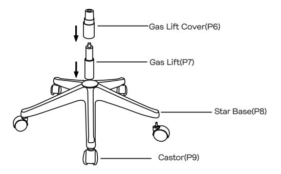
Insert 5xCastors(P9)into the Star Base(P8) as shown. Push down firmly on each castor to ensure they are fixed in position. Insert the Gas Lift(P7) into the top of Star Base(P8). Place the Gas Lift Cover(P6)over the top of the Gas Lift(P7)as shown.
