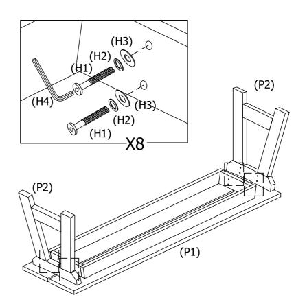
Attach bench leg frames (P2) to bench top (P1). Secure using  $8 \times 10^{1}$  x spring washers (H2) and  $8 \times 10^{1}$  washers (H3) using allen key (H4).
