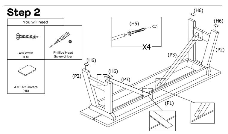
Attach 1 x stretcher (P3) to 1 x leg frame (P2) and secure using 1 x screw (H5), tightening with a phillips head screwdriver.
