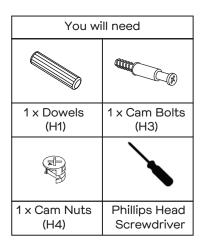
Attach 1 x Cam Bolt (H3) into Bottom Rail (P6). Insert 1 x Dowel (H1) into Top Rail (P4) and 1 x Cam Nut (H4) into Divider (P7) as shown. Rotate the cam nuts so the arrow
