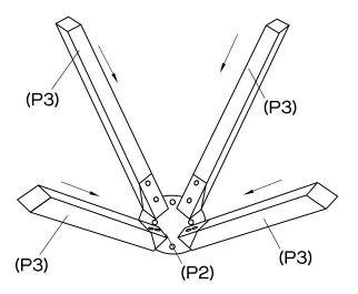
Place the  $4 \times legs$  (P3) in position of the base (P2) as shown
