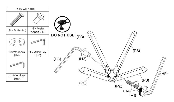
Mount the 4 x legs (P3) to the base (P2) using bolts (H1), washers (H4), metal head (H3), big allen key (H5) and small allen key (H6)
