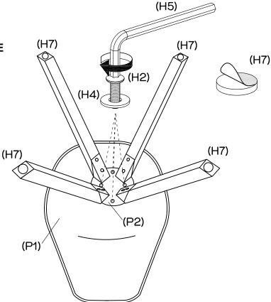
Mount the base (P2) to the seat (P1) using bolts (H2), washers (H4) and big allen key (H5). Attach felt pads (H7) to the legs.
