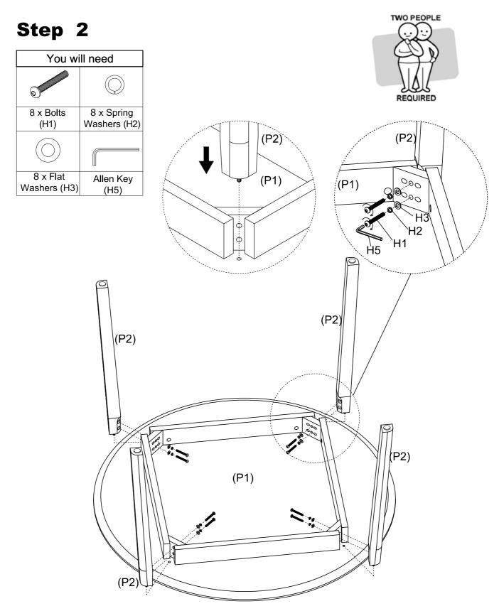
Lay top panel (P1) on to a flat soft surface as to not damage the finish. Attach each leg (P2) onto top panel (P1) with 2 x bolts (H1), 2 x spring washers (H2) and 2 x flat washers (H3). Tighten the bolts with Allen Key (H5).
