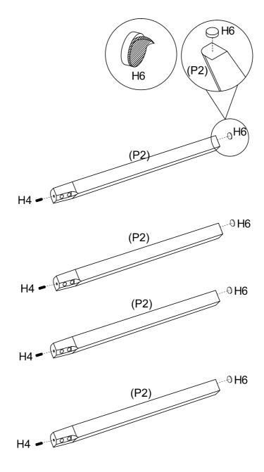
Insert each dowel (H4) into leg (P2) as shown. Attach each felt feet (H6) onto leg (P2) as shown.
