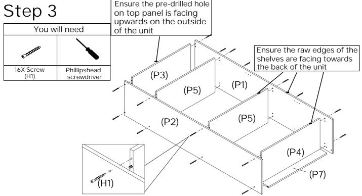
Fix Top and Bottom Panels (P3+P4), Base Panel (P7) and Fixed Shelves (P5x2) to Side Panel (P1) by tightening with Screws (H1). Repeat for Side Panel (P2).
