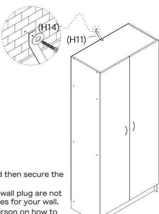
Move the unit into it's final position and then secure the Safety Strap to the wall.
