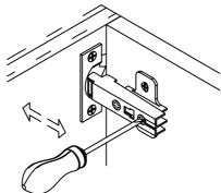
Front-to-back by slackening the hinge-arm mounting screw
