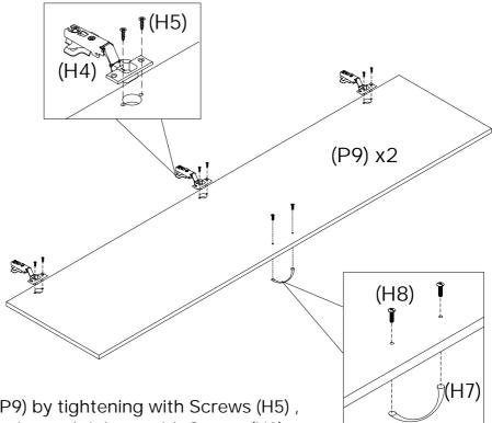
Fix Hinges (H4) to Door Panel (P9) by tightening with Screws (H5), Line Handle (H7) to pre drilled holes and tighten with Screws(H8). Repeat for Second Door Panel (P9).
