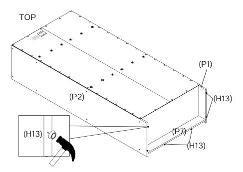
Fix Leg Studs (H13) to the bottom of Panels (P1, P2 and P7).
