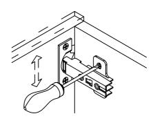
Vertical adjustment via mounting plate(via slots or, if in two pieces ,by screws)
