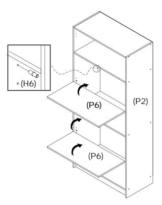
Place Shelf Supports (H6) into Side Panels (P1,P2) at preferred height. Place Adjustable Panels (P6x2) into secured shelf supports . fantasticfurniture.com.au
