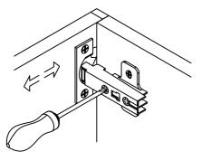
Lateral adjustment by screw adjustment
