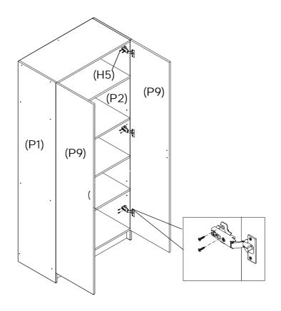
Fix Door Panels (P9x2) to Side Panels (P1, P2) using Screws (H5).
