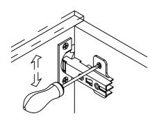
Vertical adjustment via mounting plate(via slots or, if in two pieces ,by screws)
