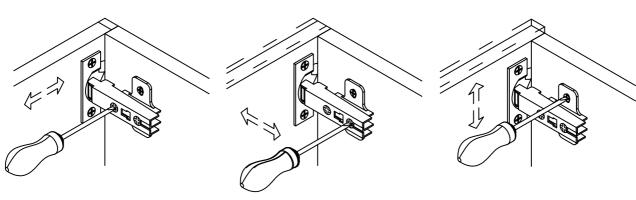
Front-to-back by slackening the hinge-arm mounting screw
