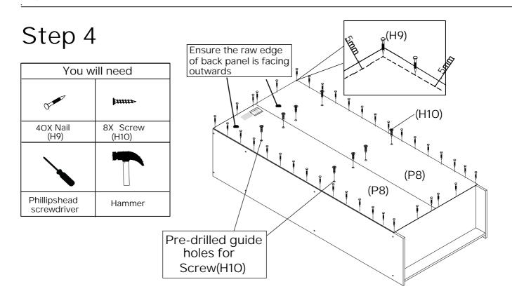
Fix Back Panel(P8) to assembled unit using Nails(H9).
