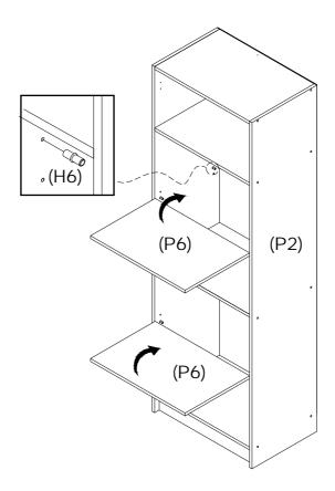
Place Shelf Supports (H6) into Side Panels (P1,P2) at preferred height. Place Adjustable Panels (P6x2) into secured shelf supports . fantasticfurniture.com.au
