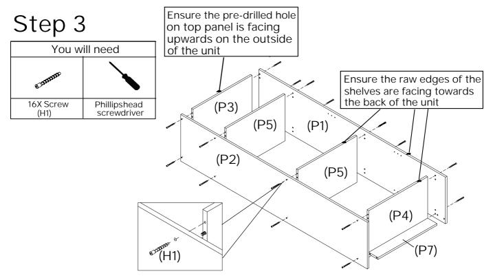
Fix Top and Bottom Panels (P3+P4), Base Pane (P7) and Fixed Shelves (P5x2) to Side Panel (P1) by tightening with Screws (H1). Repeat for Side Panel (P2).
