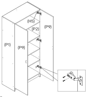
Fix Door Panels (P9x2) to Side Panels (P1,P2) using Screws (H5).
