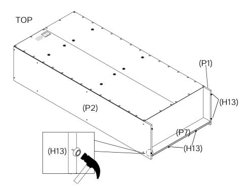
Fix Leg Studs (H13) to the bottom of Panels (P1, P2 and P7)
