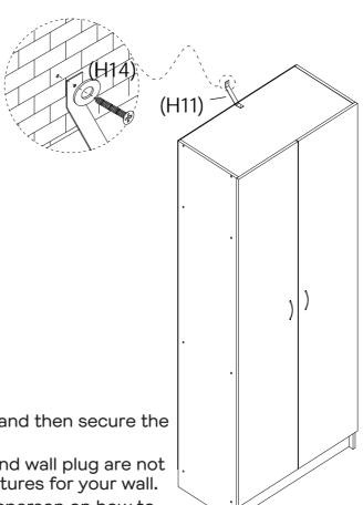
Move the unit into it's final position and then secure the Safety Strap to the wall.
