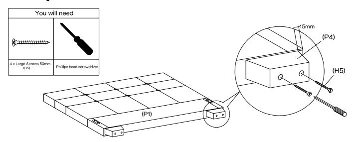
Attach 2 x legs to the bottom of the headboard (P1) with 4 x large screws (H5). The self-tapping screws provided do not require a hole to attach. Apply some pressure to the screw at the beginning, it will start to work itself into the timber frame. Keep applying the pressure as you screw until the leg is firmly attached. Repeat for the 3 other screws.
