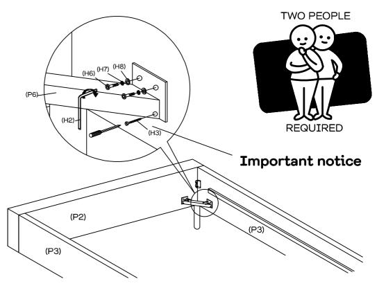
Attach the 2 x metal legs (P6) to the side rail (P3) and footboard (P2) on both corners.
