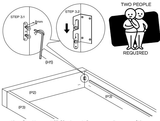
Loosen the  $4\times$  bolts on the footboard (P2) about 8mm as shown with the allen key (H1).
