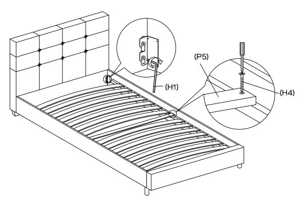
Make sure the bed frame is square, then attach the cross rail (P5) to the centre of side rails (P3) using 2x medium screws (H4). Now tighten all the bolts on the corner bracket headboard (P1) and footboard (P2).
