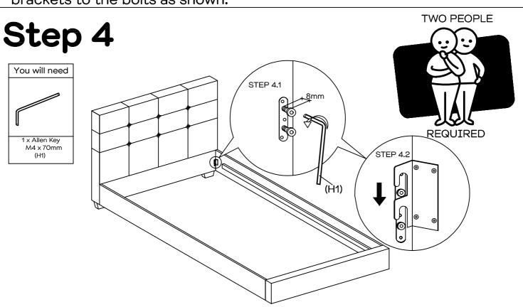
Loosen the  $4\times$  bolts on the headboard (P1) about 8mm as shown with the allen key (H1). Attach the  $2\times$  side rails (P3) to the headboard (P1) by slotting on the brackets to the bolts as shown.
