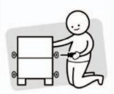
Unless instructed, do not fully tighen screws until the item is fully assembled.
