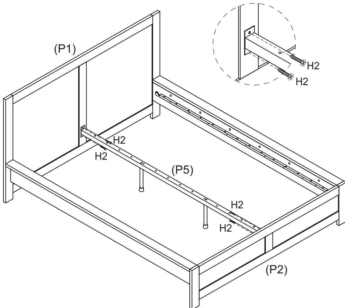
Attach Centre Rail (P5) to Bedhead (P1) and Bedfoot (P2) as shown. Then screw Centre Rail (P5) with 4 x Screws (H2).
