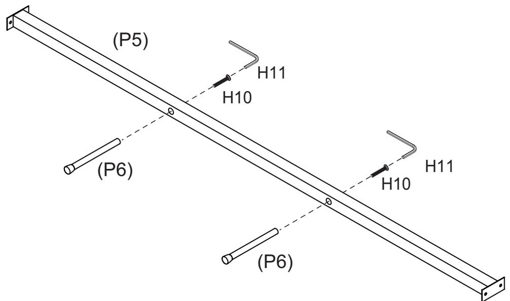
Attach 2 x Support Legs (P6) to Centre Rail (P5) with 2 x Long Bolts (H10) using Allen Key (H11).
