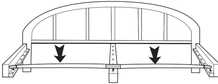
Sometimes it makes it easier to line up the hole if you press down in the middle of the slat to flatten it out.
