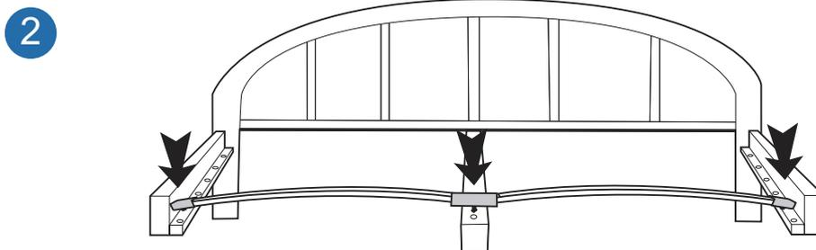
Insert the full slat into the side rail and centre rail one by one.
