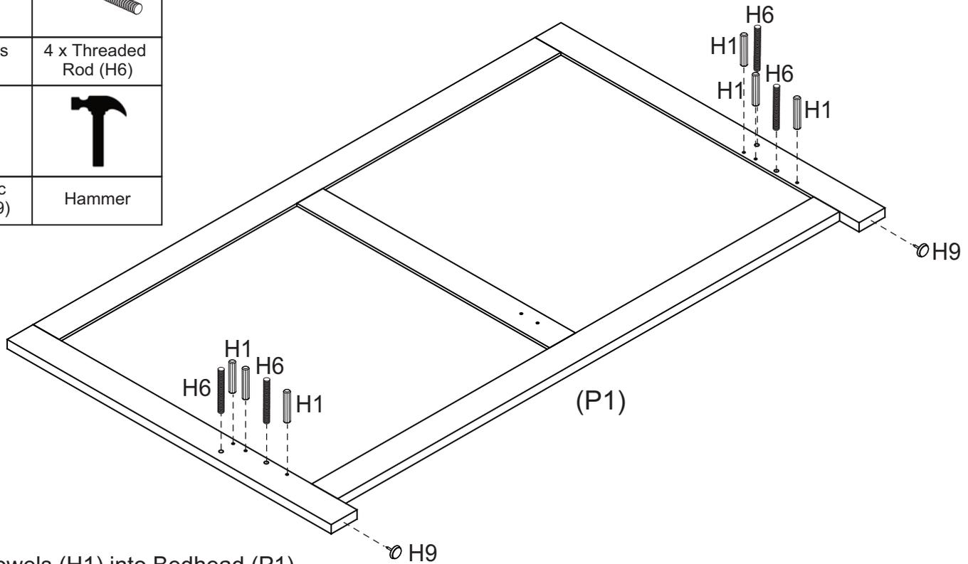
Insert 6 x Dowels (H1) into Bedhead (P1).
