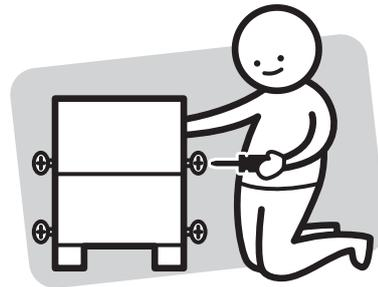
Unless instructed, do not fully tighten screws until the item is fully assembled.
