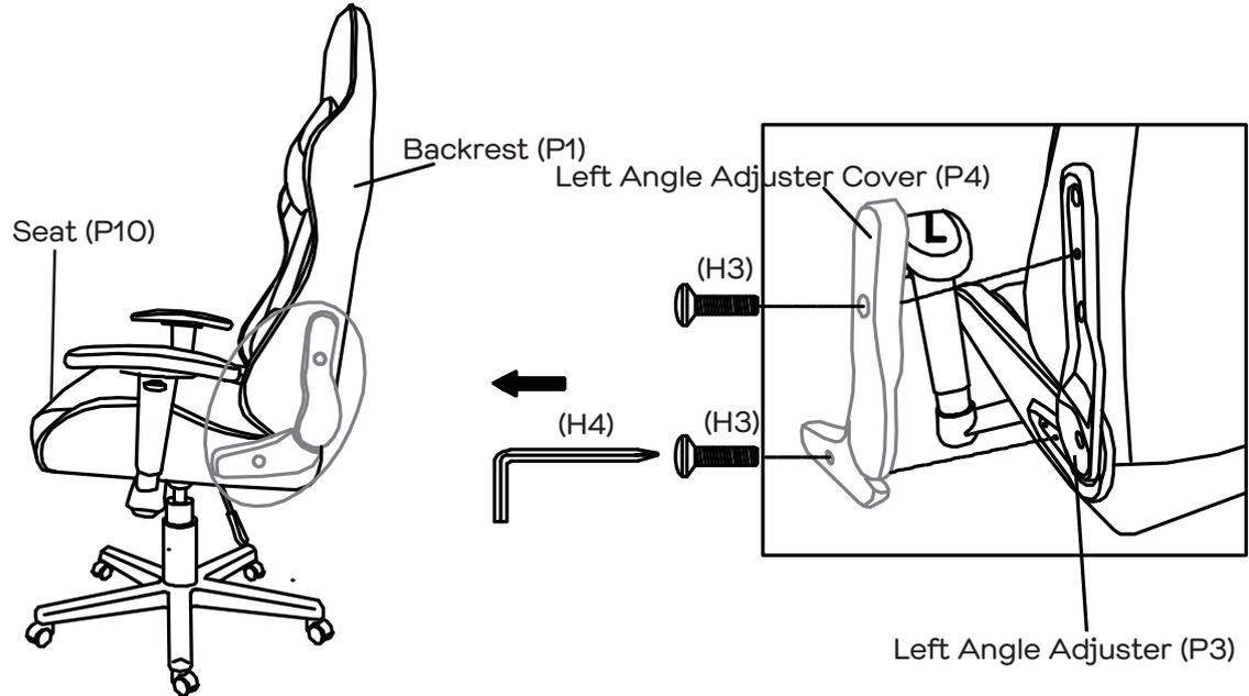
Attach Left Angle Adjuster Cover (P4) to Left Angle Adjuster (P3) by aligning the holes and securing with 2 x Small Bolts (H3) by tightening with the Allen Key (H4).
