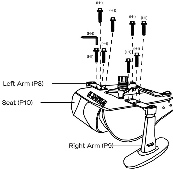
Attach the Left & Right Arms (P8&P9) to each side of the Seat (P10) as shown with 8 x Long Bolts (H1) by tightening with the Allen Key (H4). Ensure each arm is firmly secured.
