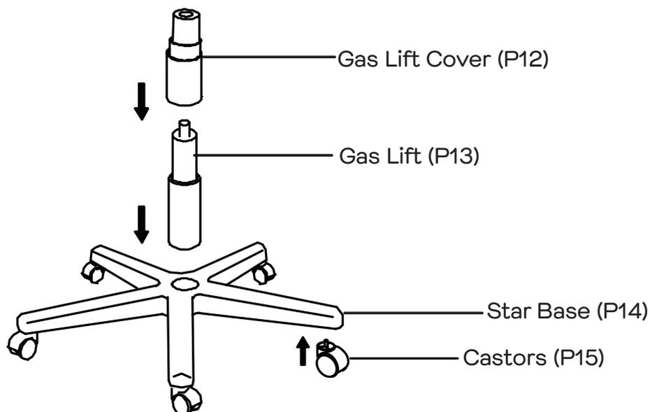
Insert 5 x Castors (P15) into the Star Base (P14) as shown. Push down firmly on each castor to ensure they are fixed in position. Insert the Gas Lift (P13) into the top of Star Base (P14). Place the Gas Lift Cover (P12) over the top of the Gas Lift (P13) as shown.
