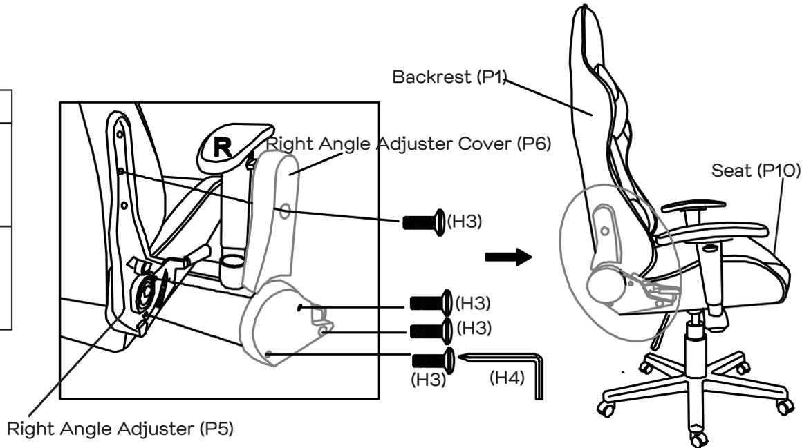
Attach Right Angle Adjuster Cover (P6) to Right Angle Adjuster (P5) by aligning the holes and securing with 4 x Small Bolts (H3) by tightening with the Allen Key (H4).
