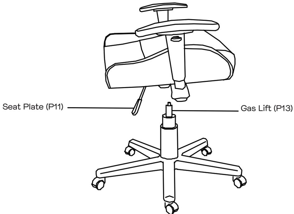
Position the center hole of the Seat Plate (P11) over the top of Gas Lift (P13). Carefully lower the Seat (P10) onto the Gas Lift (P13). Press seat down firmly. Check the connection is secure before sitting in the chair.
