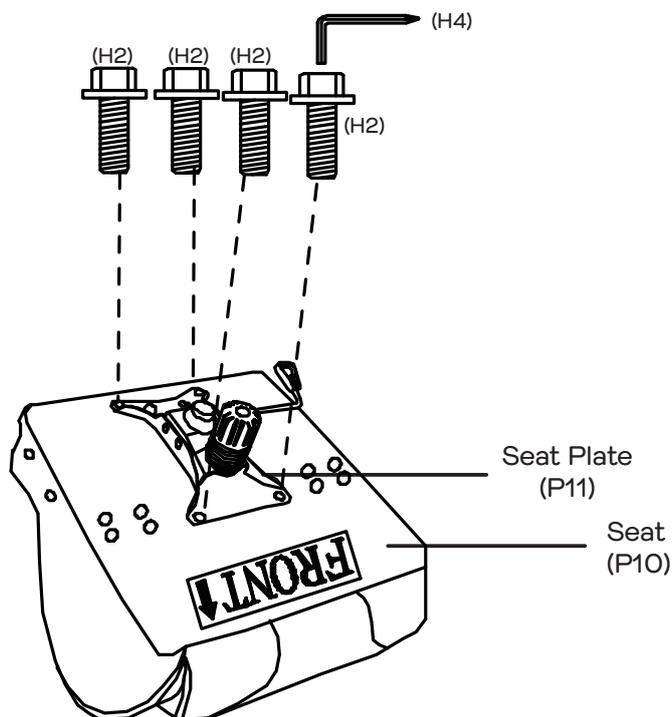
Note the front facing orientation of the Seat Plate (P11) and align the holes on the Seat Plate (P11) with the bottom of the Seat (P10) as shown. Secure the Seat Plate (P11) to the Seat (P10) with 4 x Short Bolts (H2) by tightening with the Allen Key (H4).
