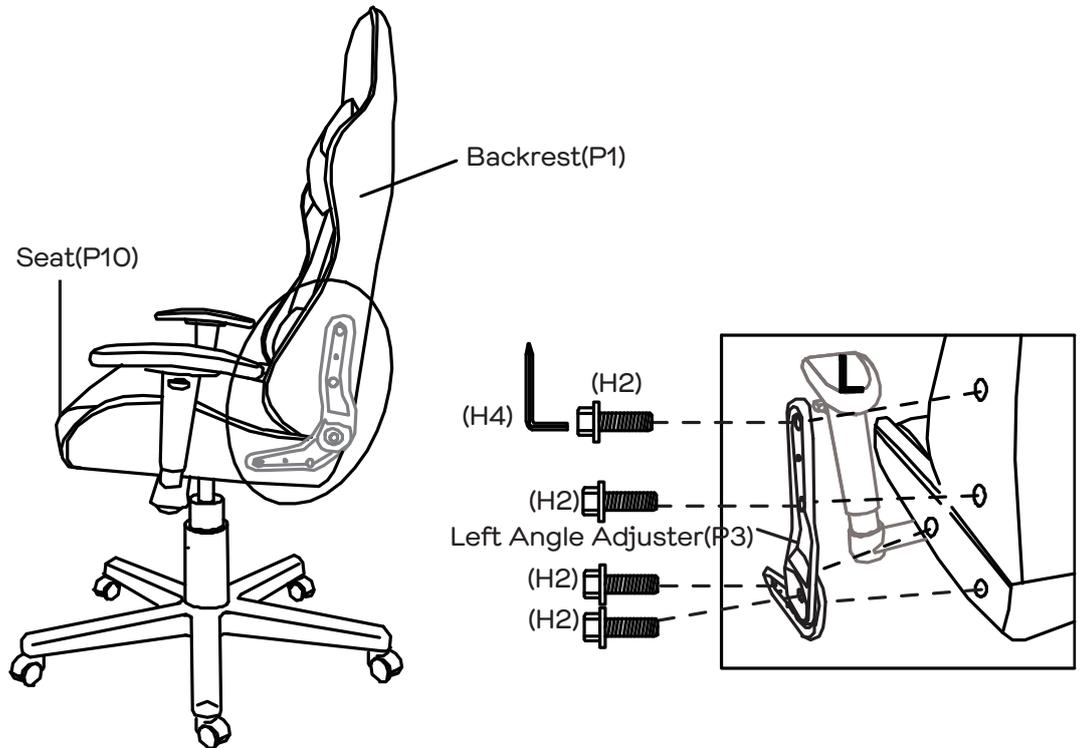
Attach Backrest (P1) to Seat (P10) by aligning the holes as shown and securing the Left Angle Adjuster (P3) with 4 x Short Bolts (H2) by tightening with the Allen Key (H4).
