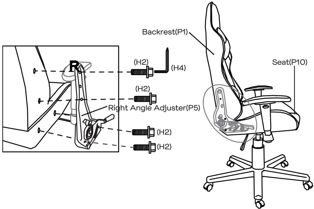
Attach Backrest (P1) to Seat (P10) by aligning the holes as shown and securing the Right Angle Adjuster (P5) with 4 x Short Bolts (H2) by tightening with the Allen Key (H4).
