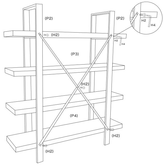
Attach Support Bars (P3 & P4) to Metal Frames (P2x2) with 5 x Short Bolts (H2) as shown by tightening with the Allen Key (H4).
