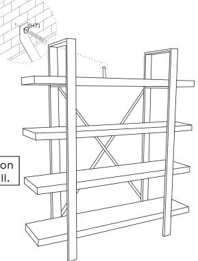
Move Bookcase to it's final position. Connect the end of Wall Strap (H6) to the wall. Make sure it is firmly attached and a snug fit.
