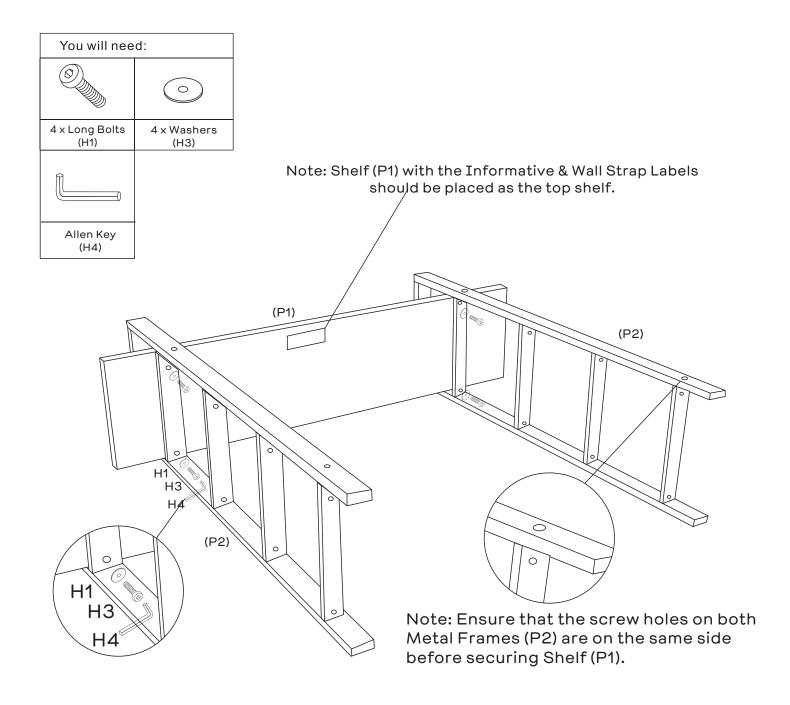
Attach Metal Frames (P2x2) to Shelf (P1) with  $4 \times$  Washers (H1) &  $4 \times$  Long Bolts (H3) as shown by tightening with the Allen Key (H4).
