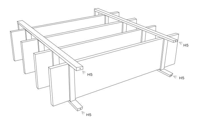
Attach  $4 \times \text{Levelling Feet}$  (H5) to the bottom of Metal Frames (P2x2) by gently screwing in. If the floor is uneven, the Levelling Feet can be adjusted as needed.
