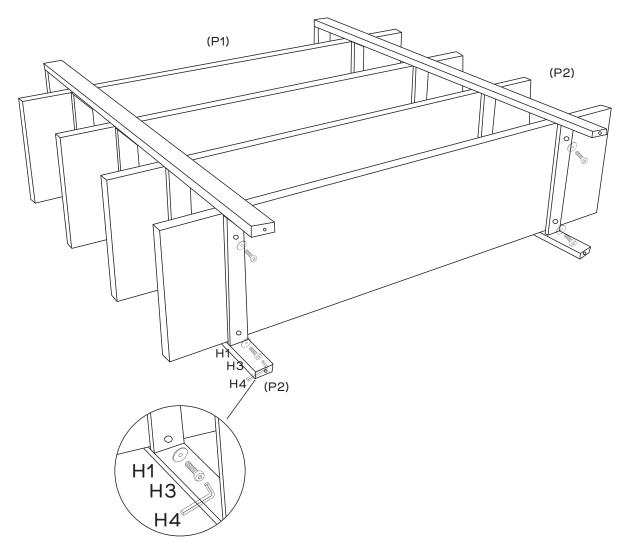
Attach Shelf (P1) to Metal Frames (P2x2) with  $4 \times$  Washers (H1) &  $4 \times$  Long Bolts (H3) as shown by tightening with the Allen Key (H4).
