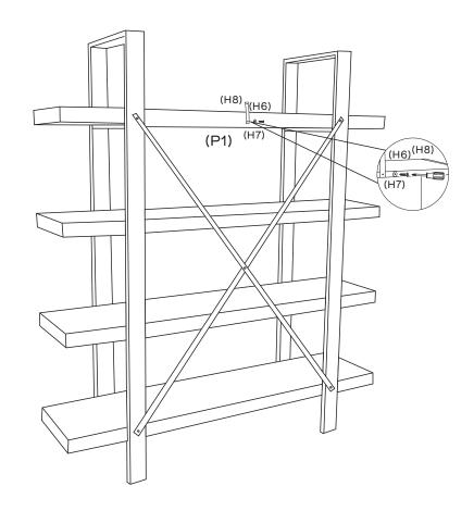
Attach Wall Strap (H8) to back of top Shelf (P1) with 1 x Washer (H7) and 1 x Screw (H6) by tightening with the Phillips Head Screwdriver.
