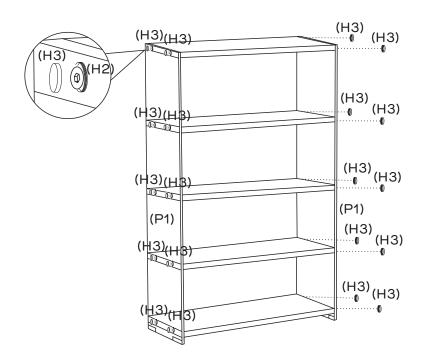
Place 20 x Bolt Caps (H3) over all Bolts (H2). Twist to tighten.
