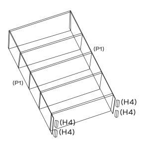
Place 4x Glass Corner Caps (H4) on the each of the bottom corners of the Glass Panels (P1x2) as shown
