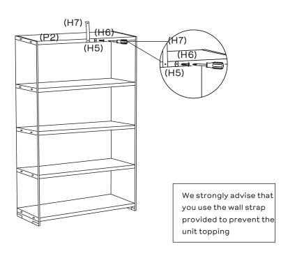
Attach Wall Strap (H7) to the back of top Shelf (P2) as shown with 1 x Washer (H5) and 1 x Screw (H6) by tightening with the Phillips Head Screwdriver.
