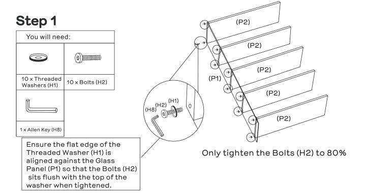
Attach Shelves (P2 x 5) to Glass Panel (P1) with 10 x Threaded Washers (H1) and 10 x Bolts (H2) by tightening with the Allen Key (H8).
