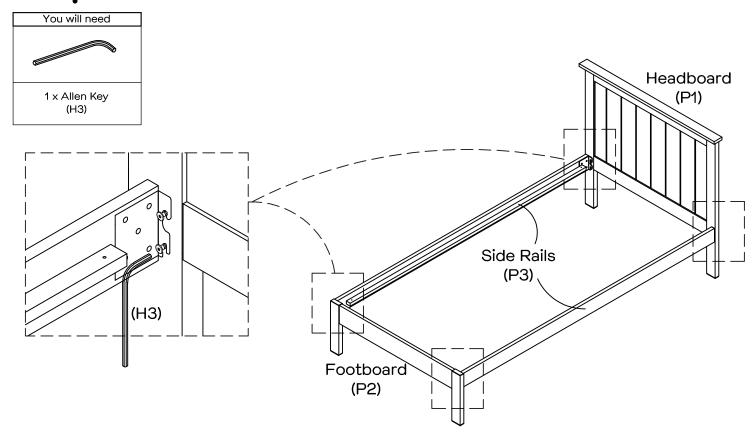
Tighten 8 x bolts (H1) by using the allen key (H3). Ensure the bolts (H1) are fully tightened.
