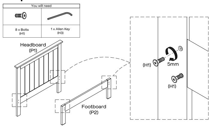
Fix 8 x bolts (H1) into the headboard & footboard (P1 & P2) about 5mm with the allen key (H3) or by hand. Do not fully tighten, as you need to slot on the side rails in the next step.
