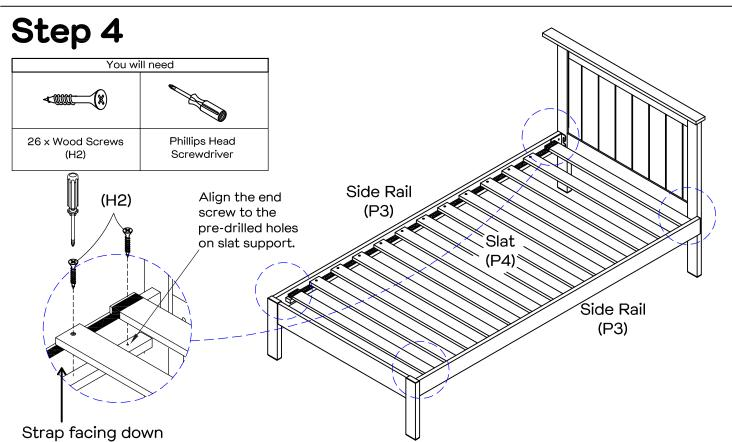
Fix the slats (P4) on to both side rails (P3) by using  $26 \times 10^{-2}$  wood screws (H2). Secure by tightening  $26 \times 10^{-2}$  wood screws (H2) with a phillips head screwdriver.
