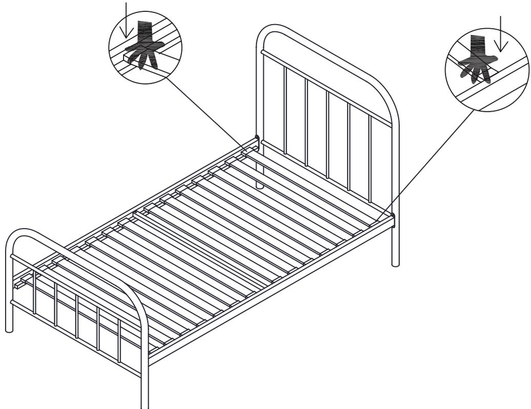
Lower the slat (P6) with the end connectors (P5) to the side rails (P3). Ensure the plastic slat caps are in place over the side rail holes and apply downward pressure until the plastic slat caps are fully inserted into the rails. Repeat for every bed slat until finished.
