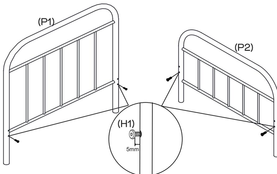
Insert 4 x short bolts (H1) into the bottom holes of the headboard (P1) and footboard (P2) using the allen key (H3). Do not fully tighten the bolts and leave a gap of 5mm as shown.
