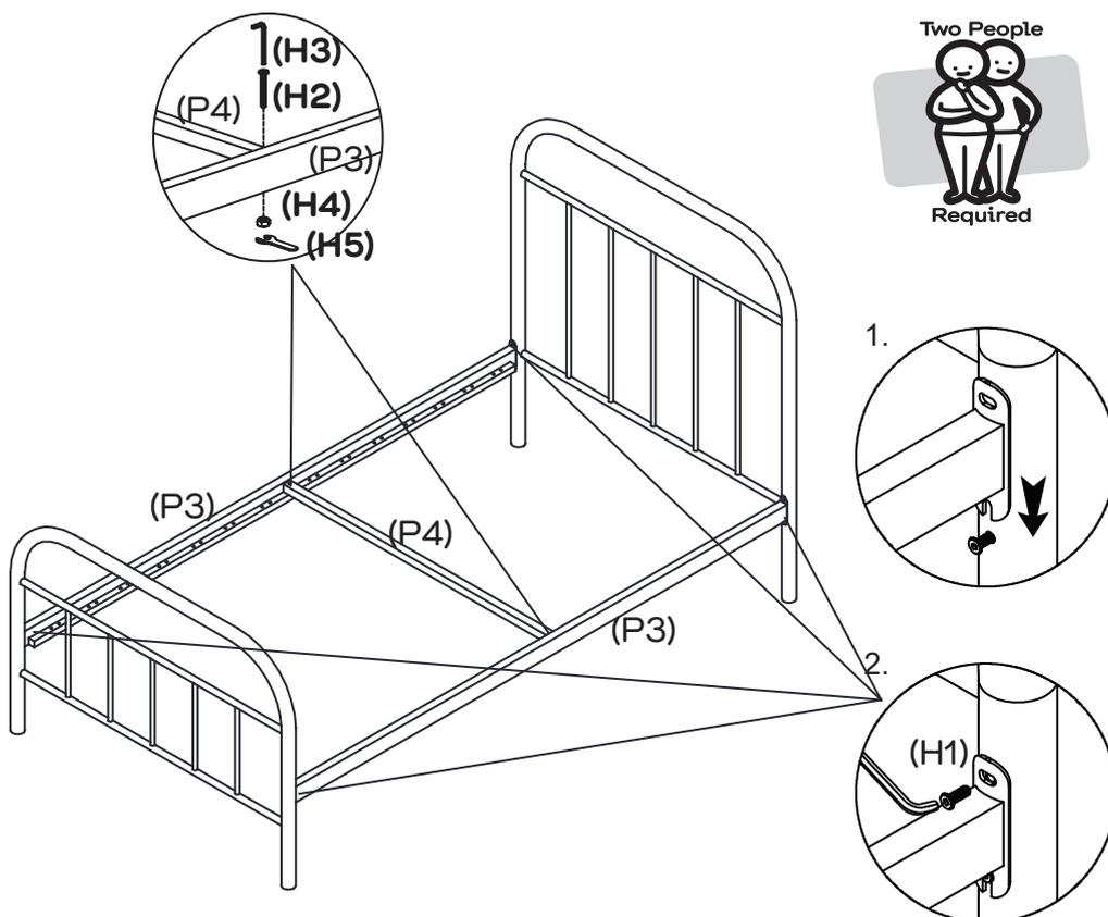
Attach the 2 x side rails (P3) to the headboard (P1) and footboard (P2). Slot the side rails onto the bolts as shown and insert 4 x short bolts (H1) into the top holes with the allen key (H3). Attach the cross bar (P4) onto the 2 x side rails (P3) using 2 x long bolts (H2) and 2 x hex nuts (H4). Tighten with the allen key (H3) and spanner (H5) as shown. Now fully tighten all bolts.
