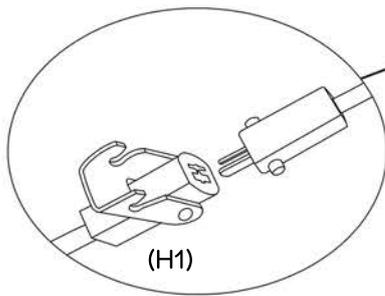
Connect the power plug (H1) to the interface of the power socket.
