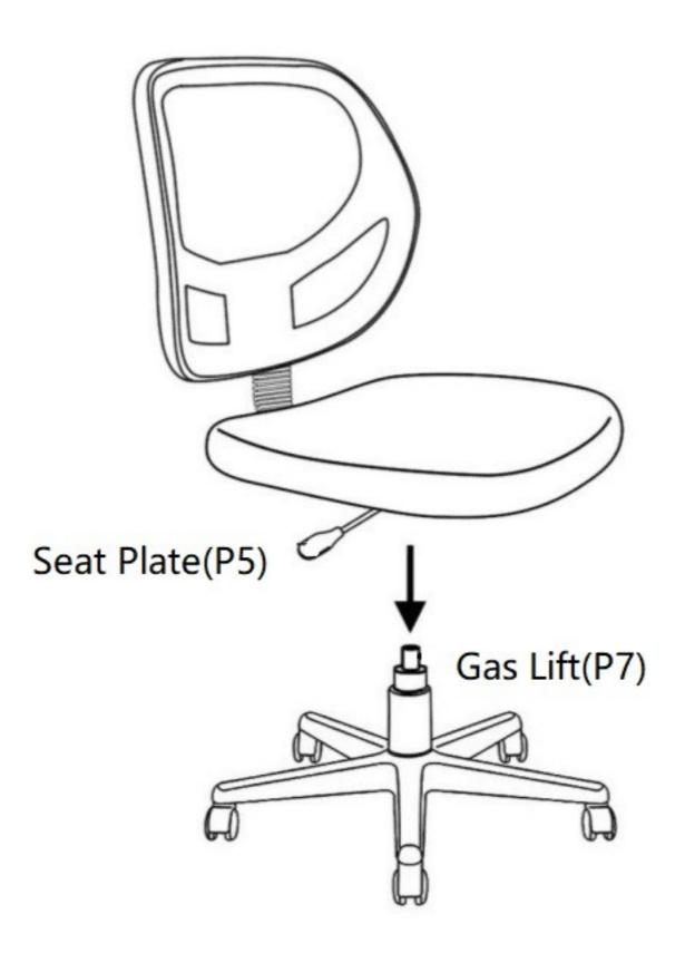
Position the centre hole of the Seat Plate(P5) over the top of the Gas Lift (P7). Carefully lower the Seat (P4) onto the Gas Lift (P7). Press seat down firmly. Check the connection is secure before sitting in the chair.
