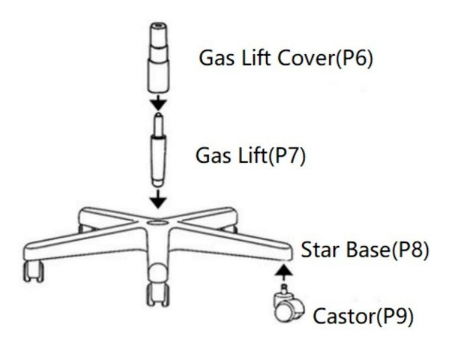
Insert 5x Castors(P9) into the Star Base(P8) as shown. Push down firmly on each castor to ensure they are fixed in position.
