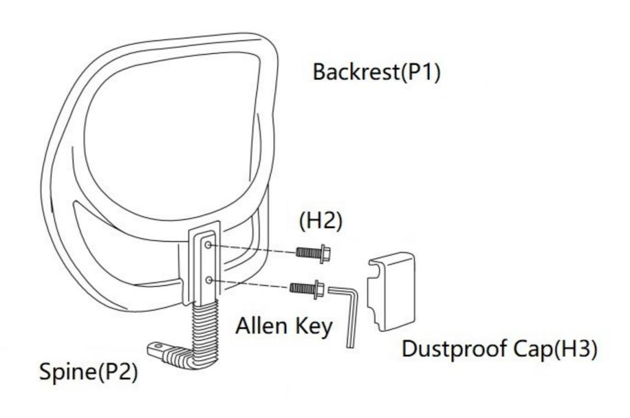
To attach the Spine (P2) to the Backrest (P1) use the Allen Key to fasten 2 x Large Bolts (H2) as shown. Ensure the bolts are tightly secured.
