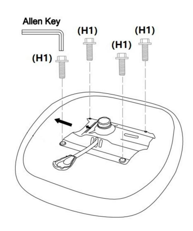
Align the holes on the Seat Plate (P5) with the bottom of the Seat (P4) and use Allen Key to fasten 4 x Small Bolts (H1) to the Seat (P4). Ensure the front of the Seat Plate (P5) is in the correct direction before securing to the base of the Seat (P4).
