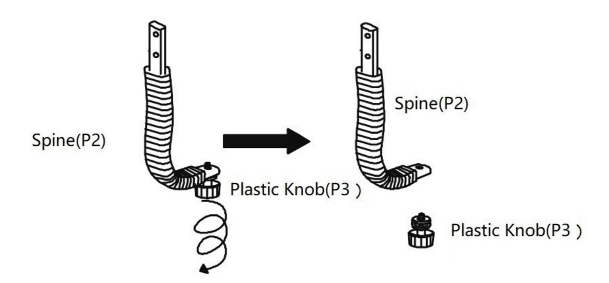
Separate the Plastic Knob (P3) from the Spine (P2) by unscrewing the Plastic Knob (P3). Carefully put aside the Plastic Knob (P3) as you will need this to secure the Spine in a later step.
