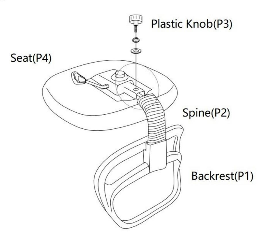
Attach the base of the Spine (P2) to the bottom of the Seat (P4) by screwing in the Plastic Knob (P3) to secure. Ensure the knob is fully tightened.
