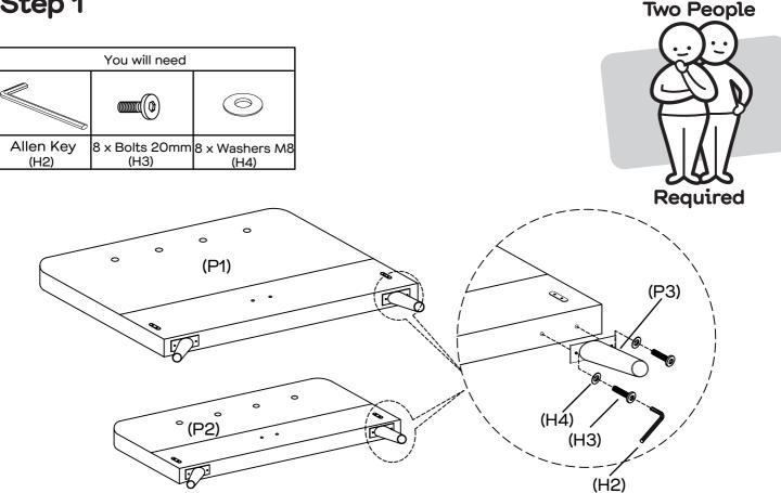
Attach legs (P3) to the bottom of headboard (P1) and footboard (P2) with 8 x bolts 20mm (H3) and 8 x washers (H4) by using allen key (H2).
