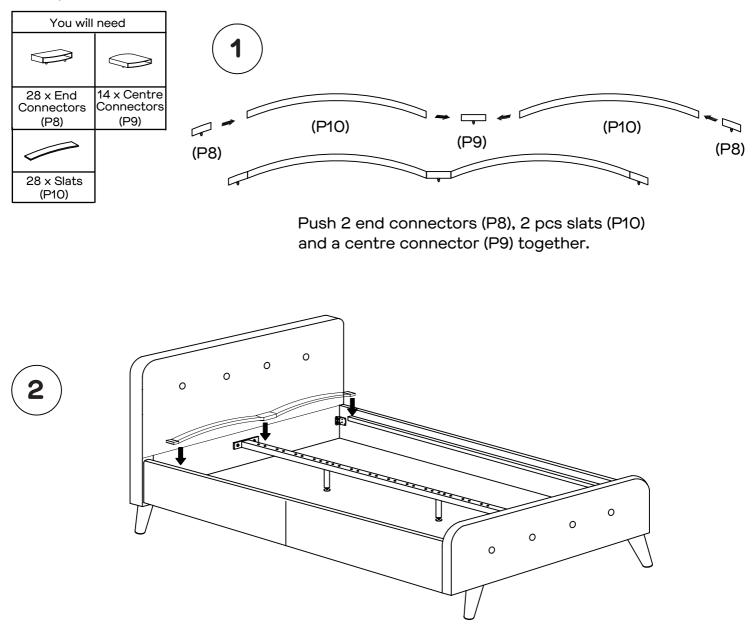
Insert the full slat into the side rail and centre rail one by one.
