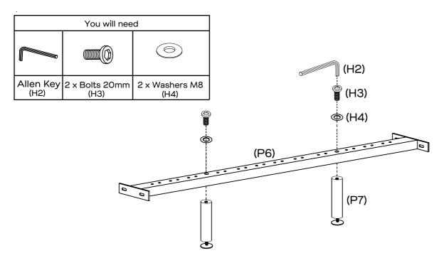
Attach the support legs (P7) to the centre rail (P6) with  $2 \times \text{bolts}$  (H3),  $2 \times \text{washers}$  (H4) by using allen key (H2).
