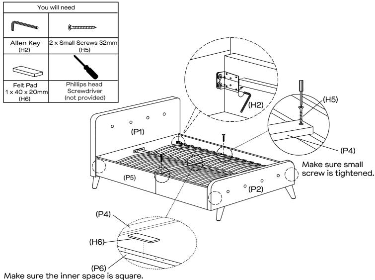
Attach the timber cross rail (P4) to the centre of side rails (P5) by using 2 x screw (H5). Then attach the felt pad (H6) to the centre of centre rail (P6). Now tighten all the bolts on the centre rail (P6) and tighten bolts on the headboard (P1) and footboard (P2).
