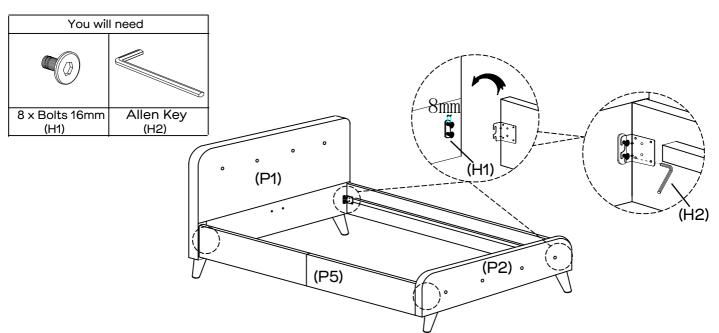
Install the bolts (H1) to the brackets by using allen key (H2) as shown, do not tighten the bolts and keep them 8mm loose. Then attach side rails (P5) to headboard (P1) and footboard (P2) by slotting the bracket on the side rails (P5) over the bolt as shown. No need to tighten bolts until step 6.
