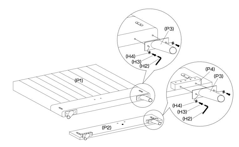
Attach 4 x legs (P3) to the bottom of headboard (P1) and footboard leg support wood (P4) with 8 x Medium Bolts (H3) and 8 x washers (H4) by using allen key (H2).
