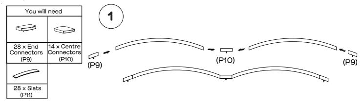
Push 2 end connectors (P9), 2 pcs slats (P11) and a centre connector (P10) together.
