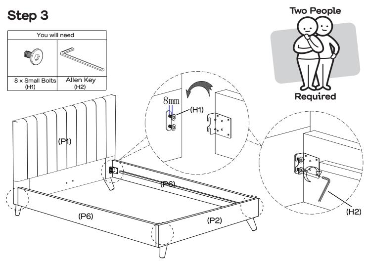
Install 8 x bolts (H1) to the brackets of the headboard (P1) and footboard (P2) by using allen key (H2) as shown, do not tighten the bolts and keep them 8mm loose. Then attach side rails (P6) to headboard (P1) and footboard (P2) by slotting the bracket on the side rails (P6) over the bolt as shown. No need to tighten bolts until step 7.
