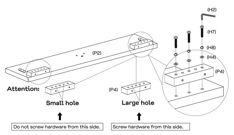
Attach 2 x footboard leg support woods (P4) to the footboard (P2) with 6 x Large Bolts (H7), 6 x washers (H4) and 6 x spring washers (H8) by using allen key (H2).
