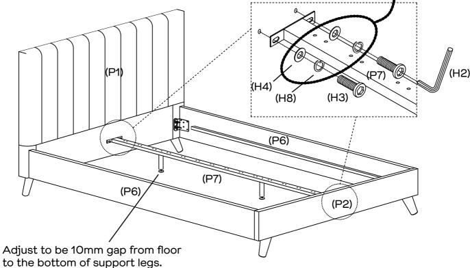
Slot the centre rail (P7) into the headboard (P1) and footboard (P2).
