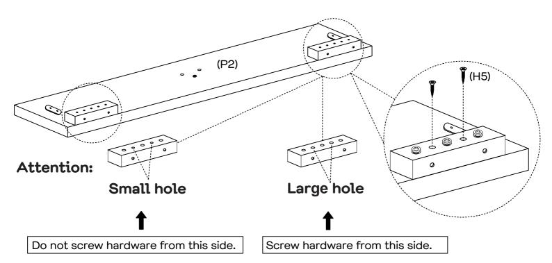
Screw the 4 x Screws (H5) by using a phillips head screwdriver (not provided).
