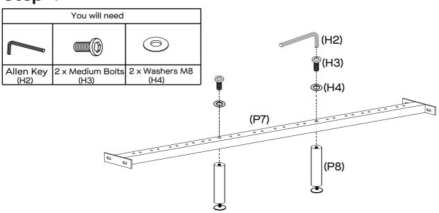
Attach 2 x support legs (P8) to the centre rail (P7) with 2 x bolts (H3) and 2 x washers (H4) by using allen key (H2).
