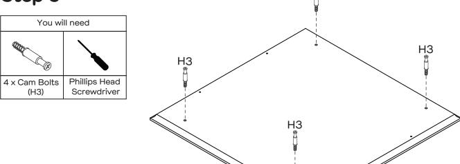
Attach 4 x Cam Bolts (H3) to Top Panel (P1) by tightening with the Phillips Head Screwdriver.
