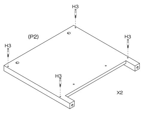
Attach 8 x Cam Bolts (H3) to Side Panels (P2x2) by tightening with the Phillips Head Screwdriver.
