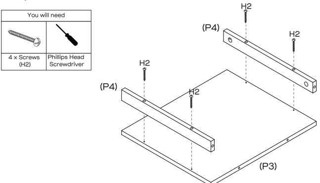
Attach Rails (P4x2) to Shelf Panel (P3) with 4 x Screws (H2) by tightening the Phillips Head Screwdriver.
