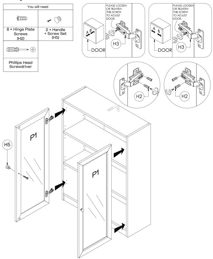
Ensure Hinges are attached to both sets of Doors as shown in Step 2. Secure Door Panels (P1x2) to left & right sides of the Bookcase with 4 x Hinges (H3) using 8 x Hinge Plate Screws (H2) by tightening with the Phillips Head Screwdriver. Attach the Handle & Screw Set (H5x2) to Door Frames (P1x2) by tightening Screws with the Phillips Head Screwdriver.
