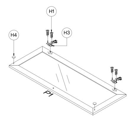
Secure  $4 \times \text{Hinges}$  (H3) to Door Panel (P1) with  $8 \times \text{Hinge}$  Screws (H1) by tightening with the Phillips Head Screwdriver.
