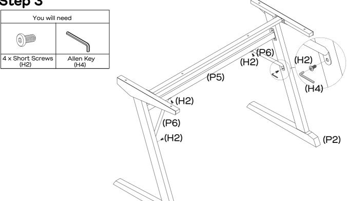
Secure Small Support Bars (P6  $\times$  2) to Support Bar (P5) and Right & Left Legs (P2 & P3) with 4  $\times$  Short Screws (H2) as shown by tightening with the Allen Key (H4).
