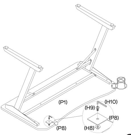
Attach Headphone Hook (P8) to the underside of the Desk Top (P1) with  $1 \times \text{Large}$  Washer (H8) and  $1 \times \text{Long}$  Bolt (H9) as shown by tightening with the Allen Key (H10). fantastic furniture.com.au
