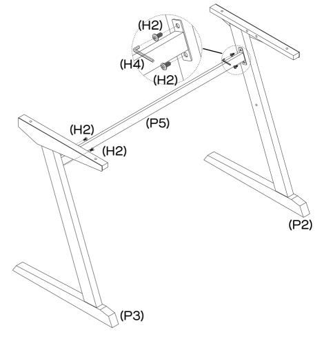
Secure Right & Left Legs (P2 &P3) to Support Bar (P5) with 4 x Short Screws (H2) as shown by tightening with the Allen Key (H4).
