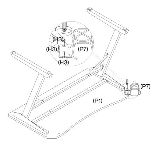
Attach Cup Holder (P7) to the underside of the Desk Top (P1) with 3  $\times$  Screws (H3) as shown by tightening with the Phillips Head Screwdriver.
