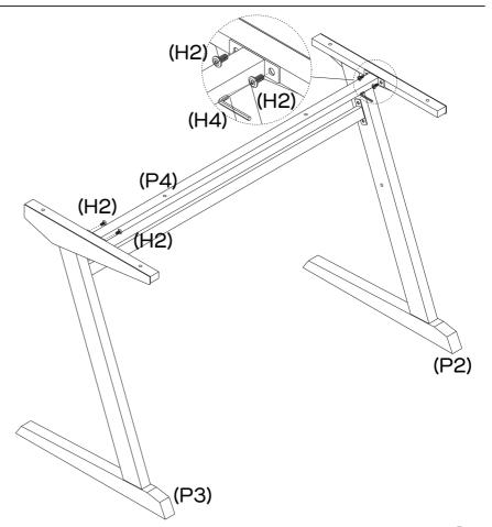
Secure Desk Top Bar (P4) to Right & Left Legs (P2 & P3) with 4 x Short Screws (H2) by tightening with the Allen Key (H4).
