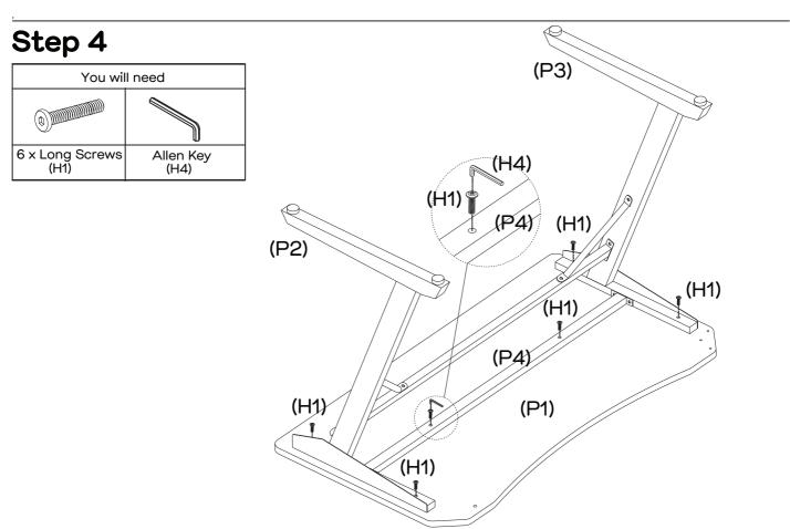
Attach Desk Top Bar (P4) and Right & Left Legs (P2 & P3) to the underside of the Desk Top (P1) with 6 x Long Screws (H1) as shown by tightening with the Allen Key (H4).
