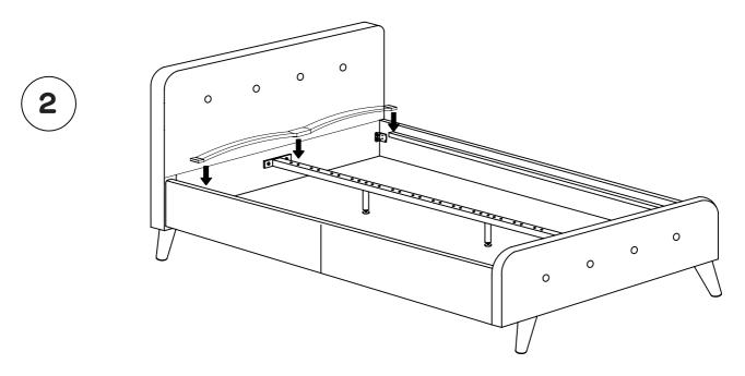
Insert the full slat into the side rail and centre rail one by one.
