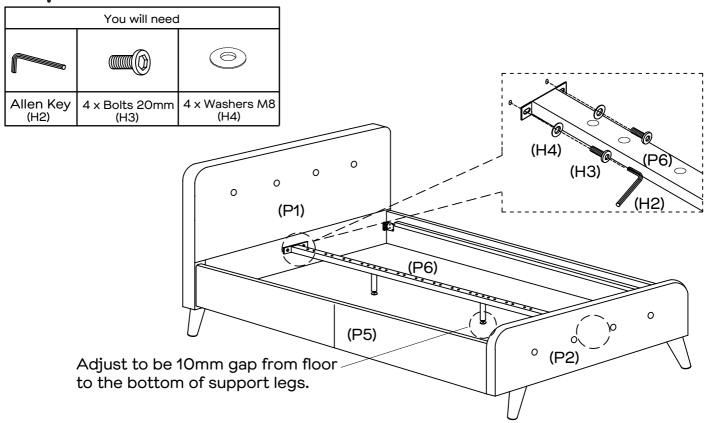
Slot the centre rail (P6) into the headboard (P1) and footboard (P2). Rotate 4 x bolts (H3) and 4 x washers (H4) using allen key (H2) to the headboard (P1) and footboard (P2). No need to tighten bolts until step 6.
