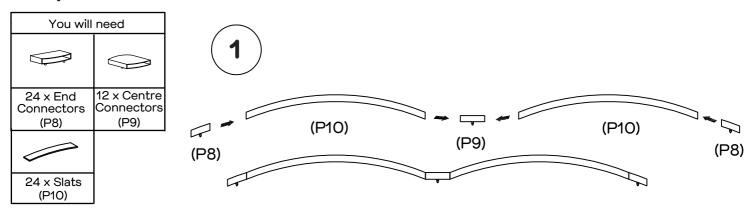
Push 2 end connectors (P8), 2 pcs slats (P10) and a centre connector (P9) together.
