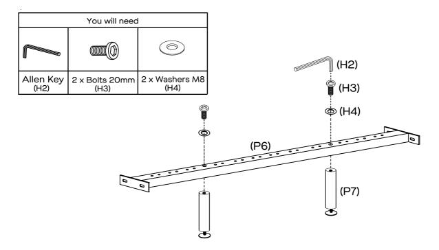
Attach the support legs (P7) to the centre rail (P6) with  $2 \times bolts$  (H3),  $2 \times washers$  (H4) by using allen key (H2).
