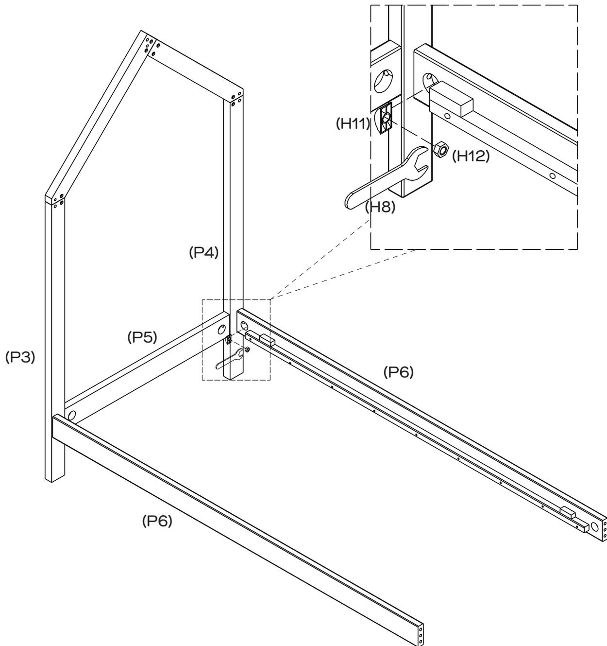
Attach the rail (P5) to the side posts (P3 & P4) by putting 2 x halfmoon nuts (H11) and 2 x hex nuts (H12) onto the 2 x locking pins (H7) as shown.
