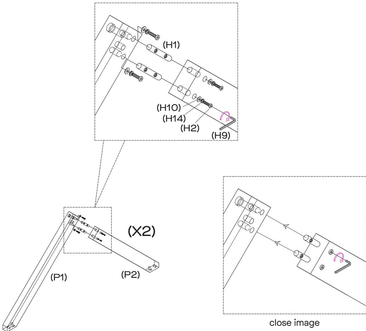
To attach the rails (P1) and (P2) together, insert 2 x steel dowels (H1) into the rails (P1 & P2). Ensure the steel dowels (H1) face the incoming bolts. Insert the 4 x short bolts (H2), the 4 x spring washers (H14) and 4 x flat washers (H10), then tighten with the allen key as shown. Repeat for the other set of panels (P1) & (P2).
