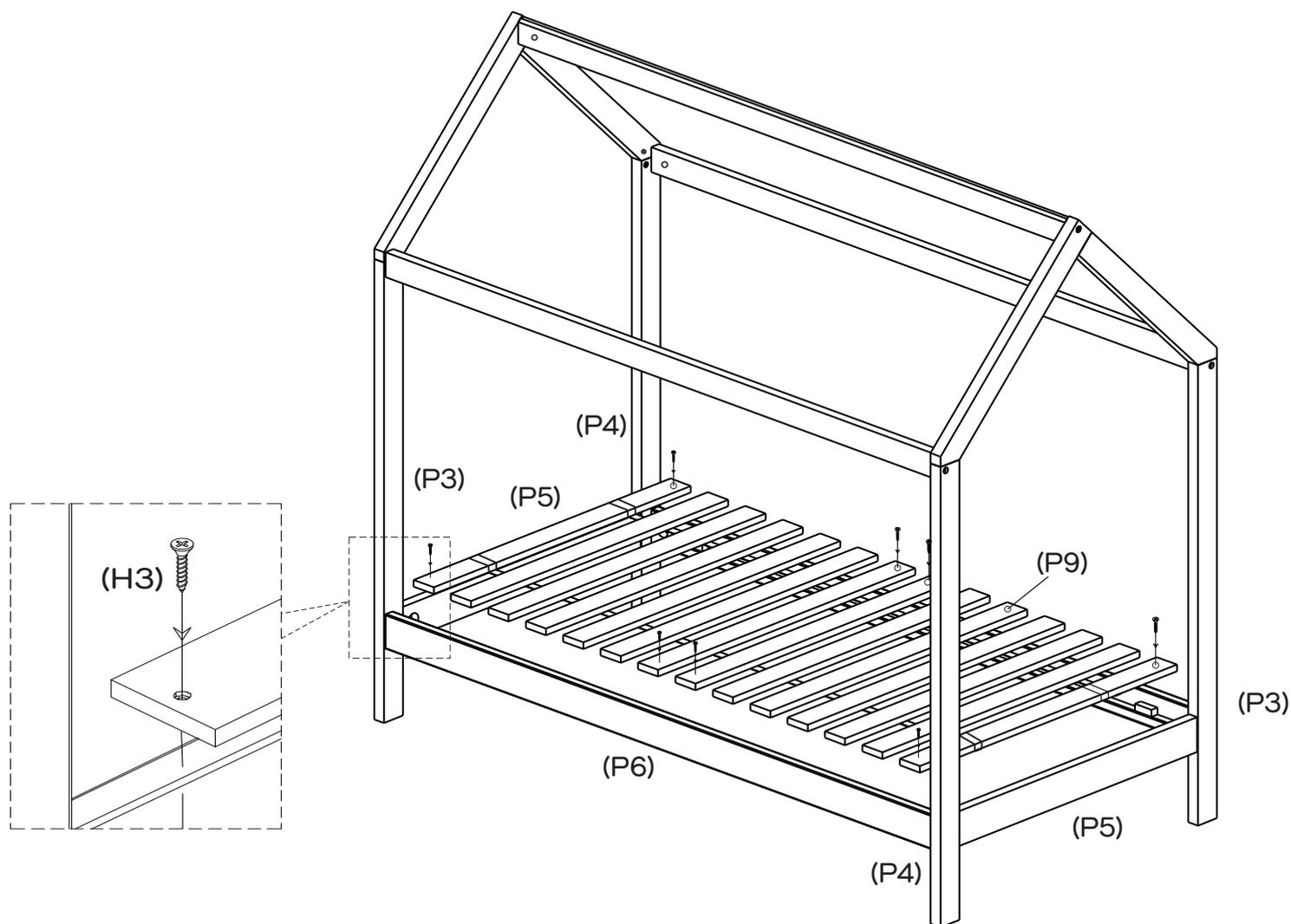
Place end slat of (P9) elastic side down on the side rail ledge, between the wooden blocks and end panel (P5).
