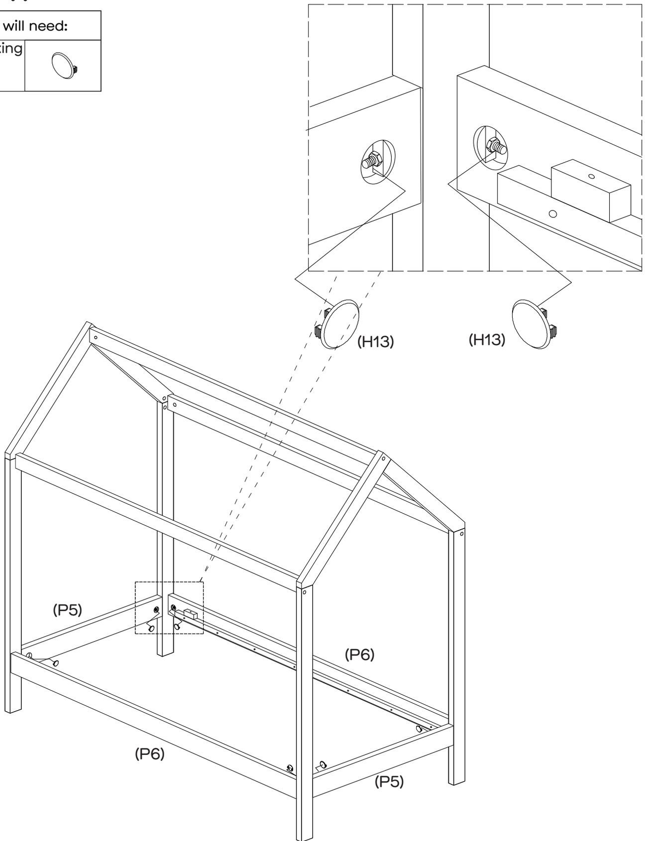
Cover the 8 holes in the side rails and end (P6 & P5) by using the 8 x locking lids (H13).
