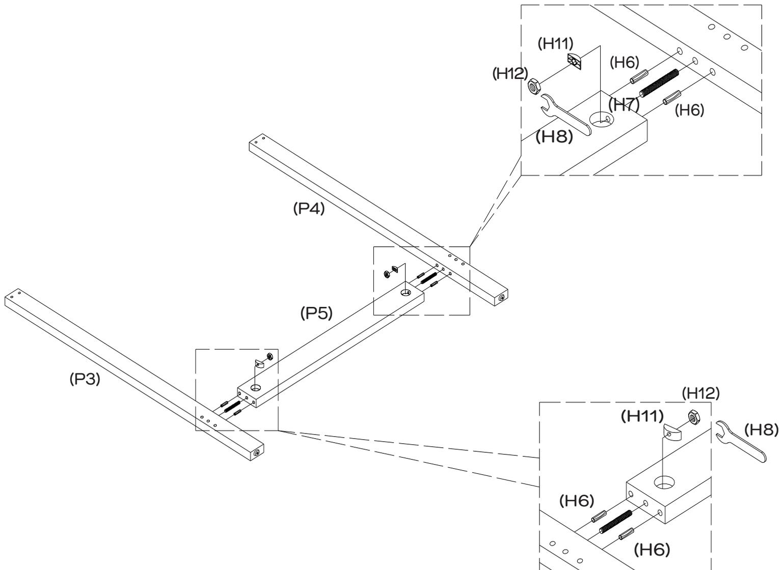
Insert 4 x wooden dowels (H6) into the side posts (P3 & P4) by hand or using a soft head mallet. Screw in 2 x locking pins (H7) into the side posts (P3 & P4) by rotating clockwise. Align the holes of the rail (P5) to the dowels (H6) and locking pins (H7) in the legs (P3 & P4). Attach the rail (P5) to the side posts (P3 & P4) by putting 2 x halfmoon nuts (H11) and 2 x hex nuts (H12) onto the 2 x locking pins (H7) as shown. Tighten the 2 x hex nuts (H12) with a spanner (H8).
