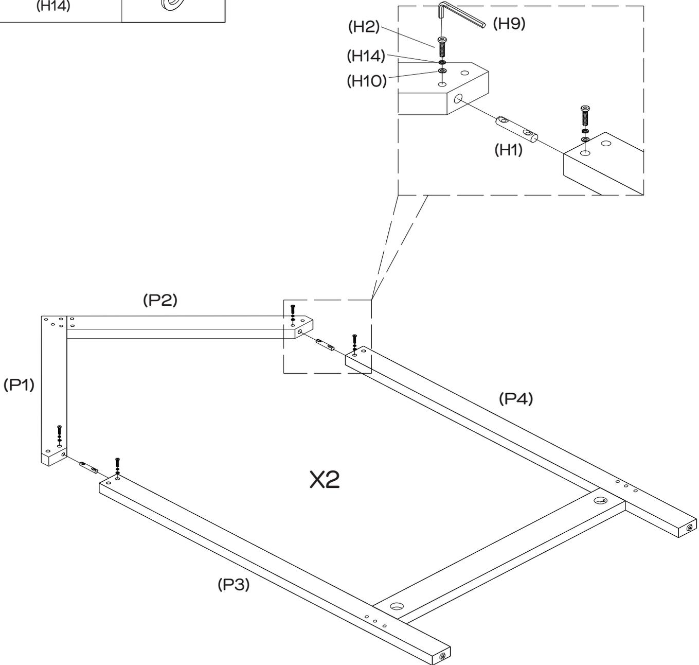
Insert 2 x steel dowels (H1) into the holes of the side posts (P3 & P4) as shown. Align panels (P1) and (P2) to the steel dowels (H1), ensuring the steel dowels (H1) face the incoming bolts (H2). Insert the short bolts (H2), the spring washers (H14) and the flat washers (H10), and tighten with the allen key (H9) as shown. Repeat for the other set of panels (P1 & P2) and (P3, P4 & P5).
