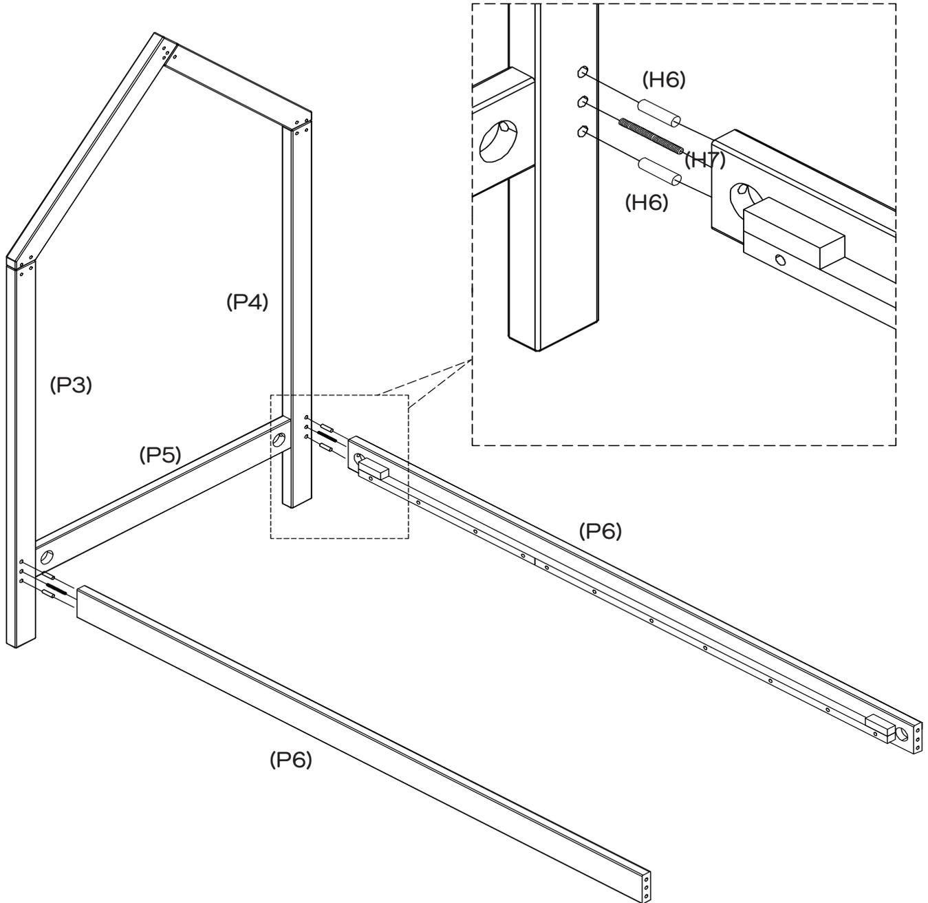
Insert 4 x wooden dowels (H6) into the side posts (P3 & P4) by hand or using a soft head mallet. Screw in 2 x locking pins (H7) into the side posts (P3 & P4) by rotating clockwise. To attach the side rails (P6) to the side posts (P3 & P4), align the holes of the rails (P6) to the dowel (H6) and locking pins (H7) in the side post (P3 & P4).
