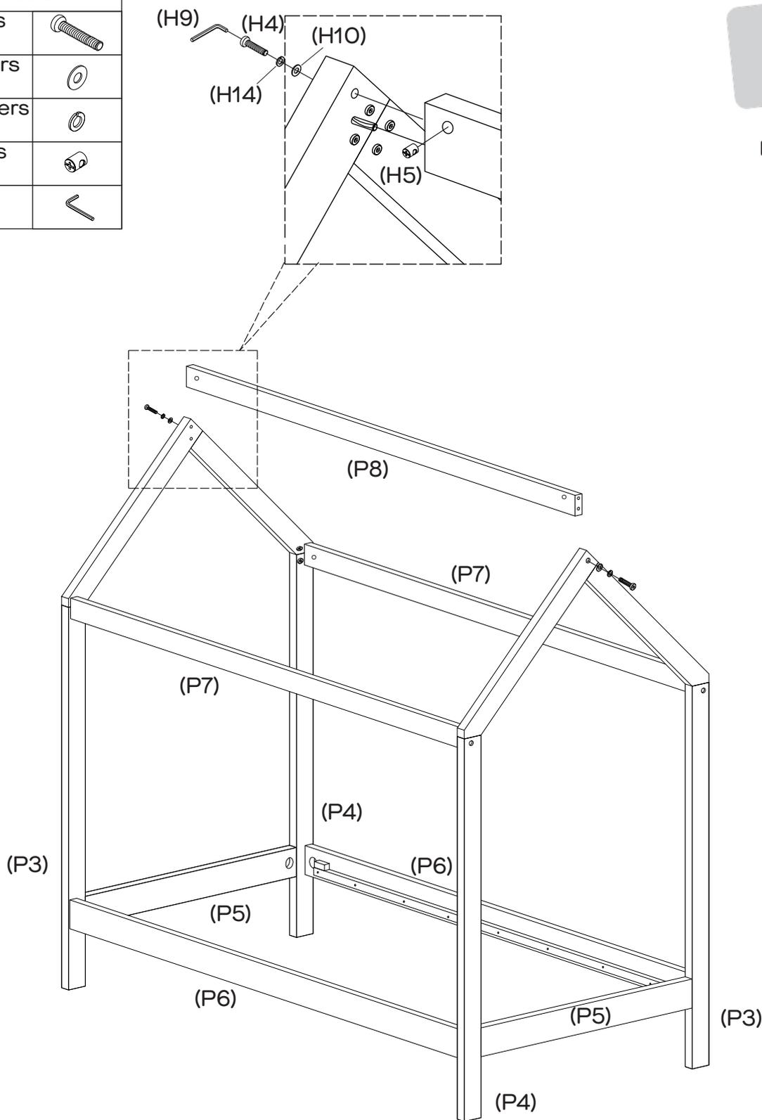
Align the top rail (P8) to the dowels on both panels (P1).
