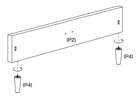
Attach 2  $\times$  footboard legs (P4) to the bottom of footboard (P2) and rotate clockwise to secure.
