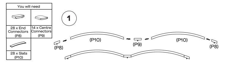
Connect 2 x End Connectors (P8), 2 x slats (P10) and a Centre Connector (P9) together as shown.
