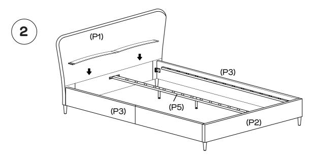
Insert the full slat into the side rails (P3) and the centre rail (P5) by pressing down firmly.
