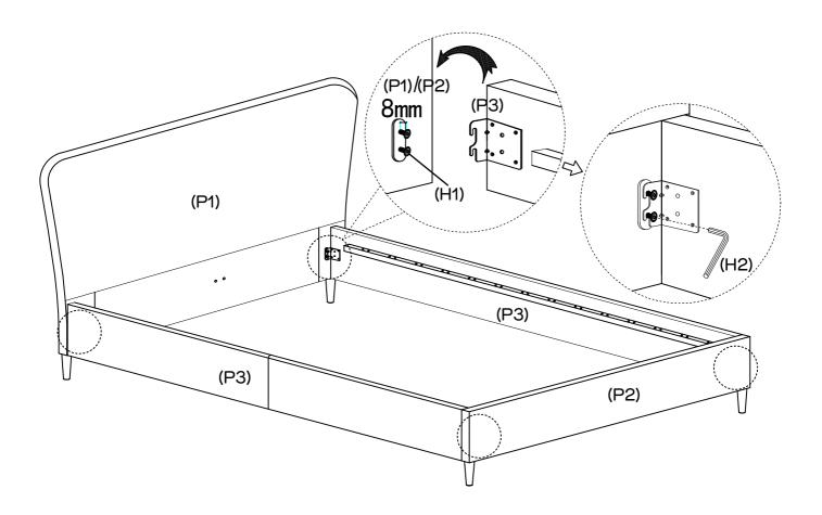
Insert 8  $\times$  big head bolts (H1) into the brackets of the headboard (P1) and footboard (P2), and tighten two thirds of the way with the allen key (H2) as shown.
