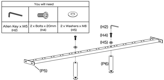
Attach 2 x support legs (P6) to the centre rail (P5) as shown using 2 x bolts (H4) and 2 x washers (H5), tightening with allen key (H2).
