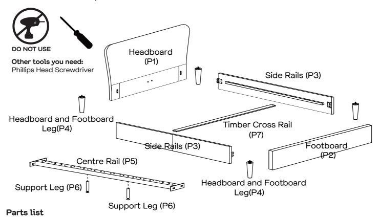
**Box 1:** Footboard (P2); 2 x Side Rails (P3); 4 x Headboard and Footboard Legs (P4); Centre Rail (P5); 2 x Support Legs (P6); Timber Cross Rail (P7); 28 x End Connectors (P8); 14 x Centre Connectors (P9); Hardware Pack
