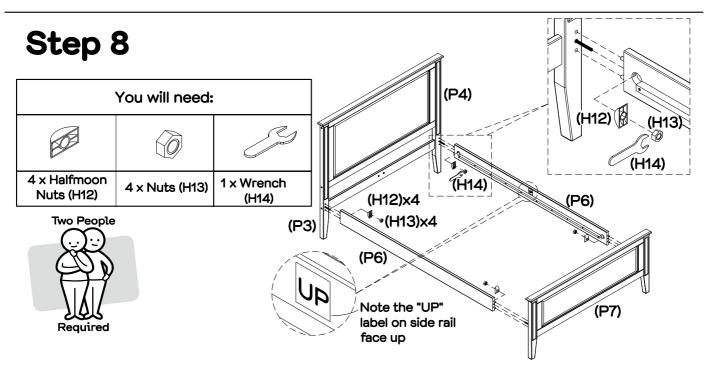
With assistance, attach left leg (P3) and footboard (P7) to the side rail (P6), insert  $2 \times \text{halfmoon}$  nuts (H12) and  $2 \times \text{nuts}$  (H13) into side rail (P6) as shown. Use the wrench (H14) to turn the nuts (H13) clockwise to fix. Repeat process for the other  $1 \times \text{side}$  rail (P6).
