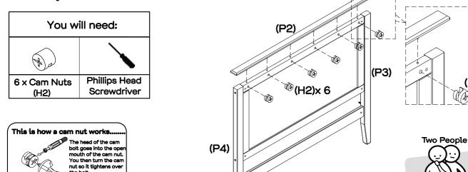
Insert  $6 \times 6 \times 6$  into headboard rail (P1), ensuring the opening of the cam nut faces incoming bolts.
