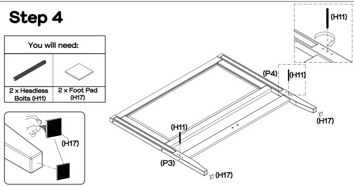
Fix 2  $\times$  headless bolts (H11) to left leg (P3) and right leg (P4), turn clockwise to lock in position.
