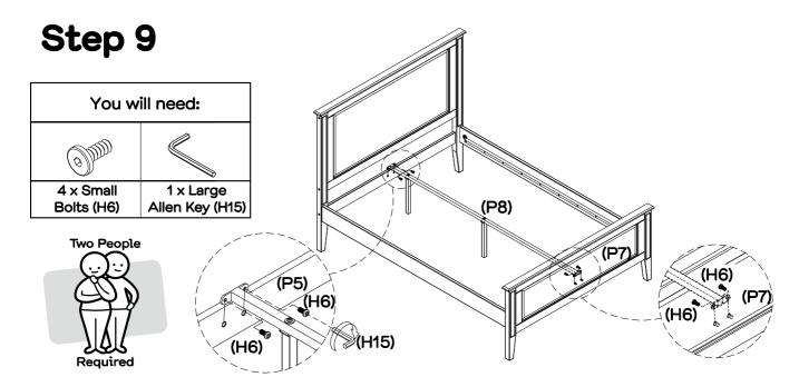
With assistance, attach the centre rail (P8) to the headboard rail (P5) and footboard (P7) using 4 x small bolts (H6) tightening by turning clockwise using large allen key (H15). You may now fully tighten the bolts attaching the side rails (P6) to the left leg and right leg (P3, P4) and footboard (P7).
