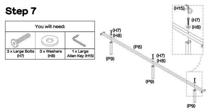
Attach 3  $\times$  centre legs (P9) to the centre rail (P8) using 3  $\times$  washers (H8) and 3  $\times$  large bolts (H7). Tighten the bolts by turning clockwise using large allen key (H15).
