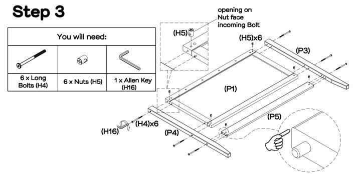
Insert  $6 \times \text{nuts}$  (H5) into the headboard rail (P5) and headboard core (P1) as shown. Ensure the opening of the nut faces incoming bolts.
