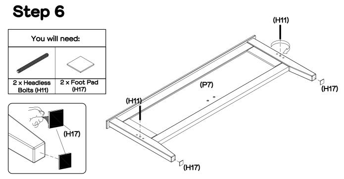
Fix 2  $\times$  headless bolts (H11) to leg, turn clockwise to lock in position. Attach 2  $\times$  foot pads (H17) to leg.
