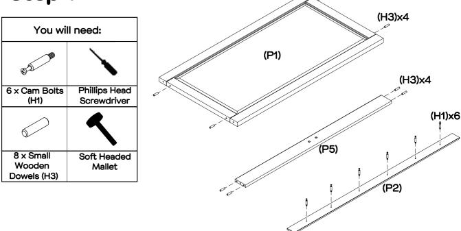
Insert 8 x small wooden dowels (H3) into the headboard core (P1) and headboard rail (P5) as shown.
