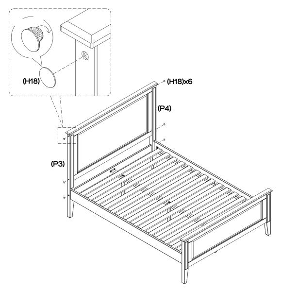
Attach  $6 \times PVC$  stickers (H18) to left leg (P3) and right leg (P4).
