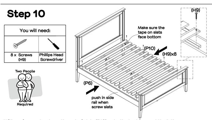
With assisance, lay down the set of slats (P10) onto the bed frame. Attach the slats (P10) to the  $2 \times \text{side}$  rails (P6) using  $8 \times \text{screws}$  (H9), tightening with a phillips head screwdriver.
