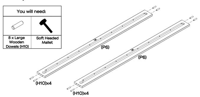
Insert 8 x large wooden dowels (H10) into the Side Rail (P6) as shown.
