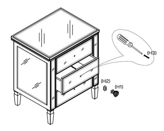
Attach the  $3 \times$  handles (H1) to the outside of the drawer using  $3 \times$  washer (H2) and  $3 \times$  bolts (H3) as shown.
