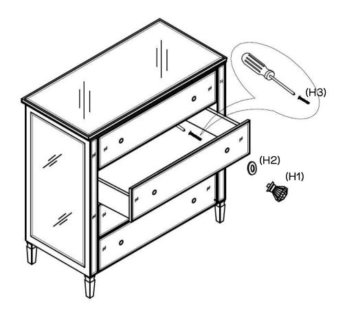
Attach the 8 x handles (H1) to the outside of the drawer using 8 x washer (H2) and 8 x bolts (H3) as shown.
