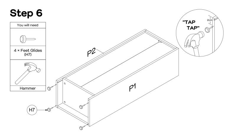
Secure 4 x Feet Glides (H7) to the bottom of Left & Right Side Panels (P1&P2) with the Hammer. Ensure the feet glides are evenly spaced, approximately 2cm from the end of each panel.
