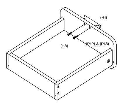
Attach the 2 x Handles to the Drawer Fronts (P12 & P13) with 2 x Handle Screws (H8), by tightening with a Phillips Head Screwdriver.
