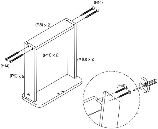
Attach the Drawer Back Panels (P8) to the Drawer Side Panels (P9 & P10) with 8 x Drawer Screws (H14), by tightening with a Phillips Head Screwdriver. Before securing, ensure the Drawer Base Panel (P11) lines up with the grooves the whole way around the drawer.
