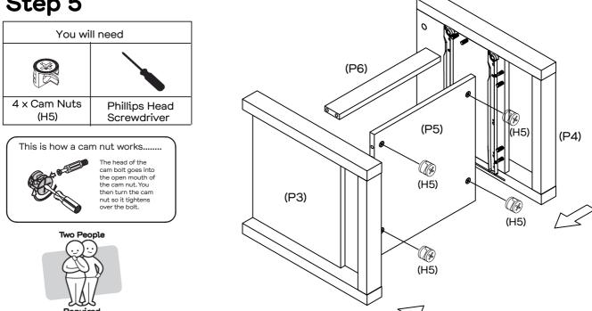
Insert 4 x Cam Nuts (H5) into the Base Panel (P5).
