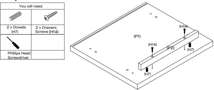
Attach Support Panel (P2) to the Top Panel (P1) with  $2 \times 1$  Dowels (H7) and  $2 \times 1$  Drawer Screws (H14), by tightening with the Phillips Head Screwdriver.
