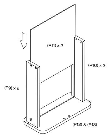
Slot in the Drawer Base Panel (P11) into the grooves of panels (P9, P10, P12 & P13) as shown.
