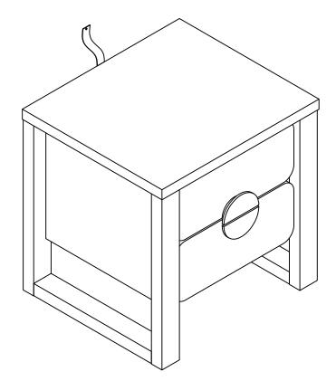
Move the unit to the final position, and attach the safety strap to the wall securely. Make sure it is firmly attached and snug fit.
