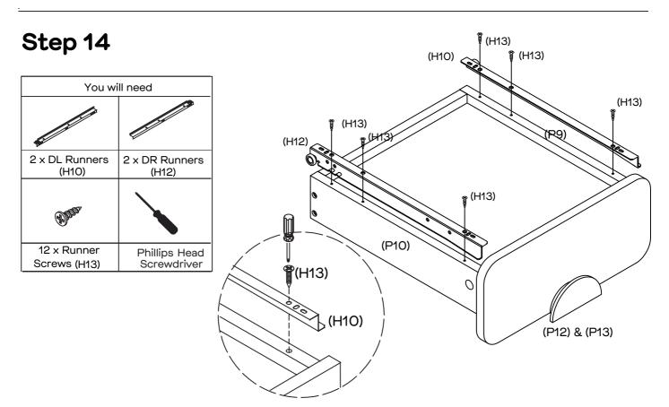
Attach 1 x DL Runner (H10) to the bottom of Drawer Side Panel L (P9) and 1 x DR Runner (H12) to the bottom of Drawer Side Panel R (P10) with 6 x Runner Screws (H5) by tightening with the Phillips Head Screwdriver. Repeat process for the remaining drawer.
