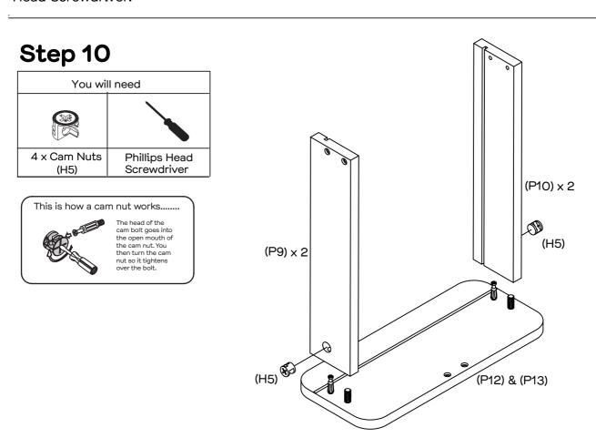
Insert 4 x Cam Nuts into the Drawer Side Panels (P9 & P10). Rotate the Cam Nuts so the arrows point towards the incoming cam bolts. Attach the Drawer Front Panels (P12 & P13) to the Drawer Side Panels (P9 & P10), by tightening Cam Nuts with the Phillips Head Screwdriver.
