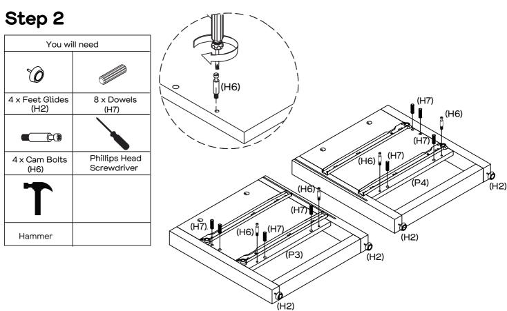
Insert 4 x Cam Bolts (H6) into the Left Side Panel (P3) and Right Side Panel (P4), by tightening with a Phillips Head Screwdriver.
