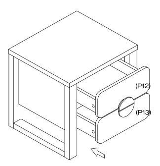
Insert the assembled drawers into the corresponding compartments as shown. Ensure the drawers slide easily along the rails.
