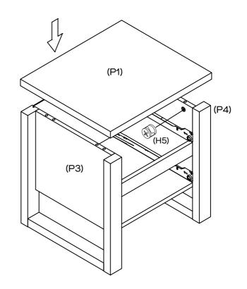
Insert 4 x Cam Nuts into Left Side Panel (P3) and Right Side Panel (P4).
