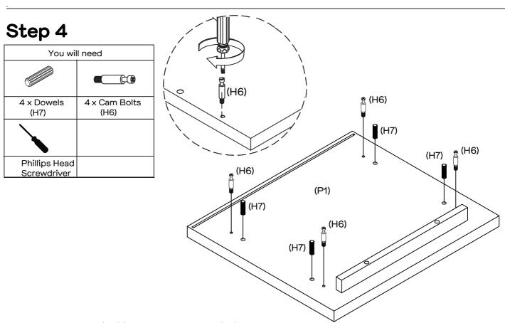
Insert 4 x Dowels (H7) into the Top Panel (P1).
