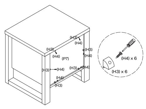
Secure Back Panel (P7) in place with 6 x Wedges (H3) using 6 x Wedge Screws (H16) by tightening with the Phillips Head Screwdriver.
