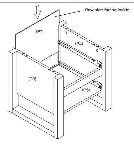
Slot the Back Panel (P7) into the grooves of panels (P3, P4 & P5) as shown.
