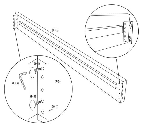
Attach the 4  $\times$  brackets (H4) to the ends of the side rails (P3) as shown. Screw in 2  $\times$  bolts (H1) into each bracket with the allen key (H3). Ensure to fully tighten all bolts.
