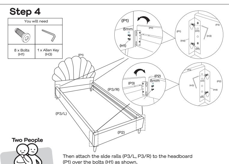
Then attach the side rails (P3/L, P3/R) to the footboard (P2) over the bolts (H1).
