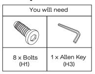
Install 4 x bolts (H1) into the headboard (P1) and footboard (P2) by using the allen key (H3) as shown, do not fully tighten the bolts and keep them 8mm loose.
