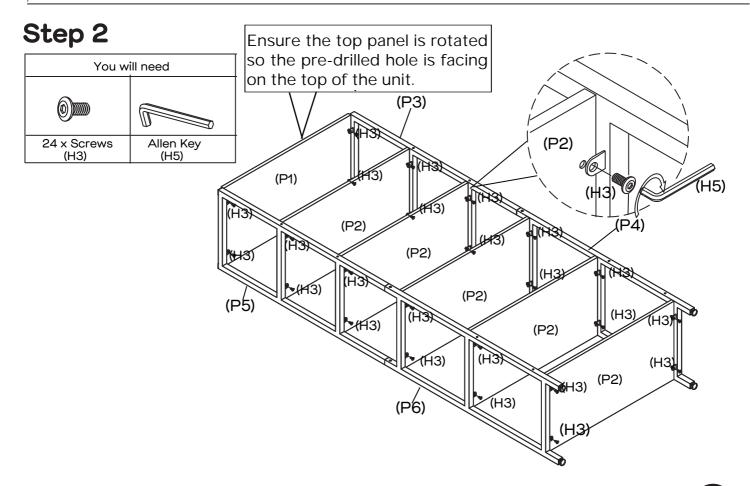
Secure Top Panel (P1) and Shelf Panels (P2x5) to Top & Lower Left/Right Frames (P3,P4,P5&P6) with 24 x Screws (H3) as shown by tightening with the Allen Key (H5).
