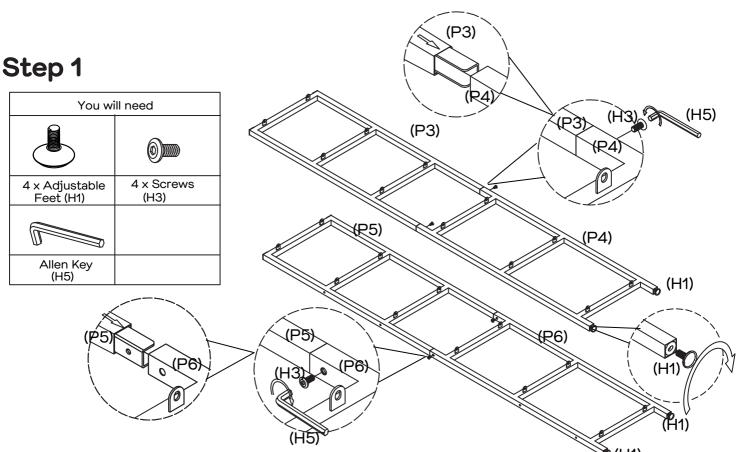
Attach Top & Lower Left Frames (P3&P4) as shown with 2 x Screws (H3) by tightening with the Allen Key (H5).
