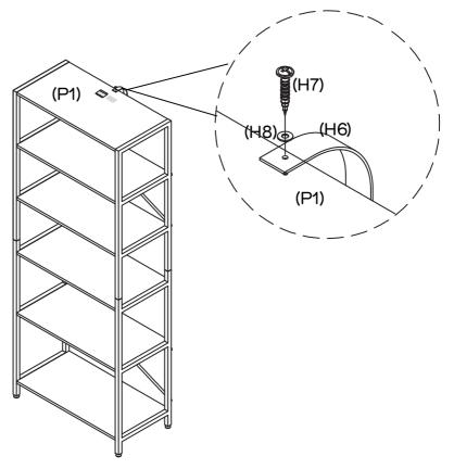
Attach the Wall Strap (H6) to Top Panel (P1) with 1 x Washer (H8) and 1 x Wall Strap Screw (H7) by tightening with the Phillips Head Screwdriver.
