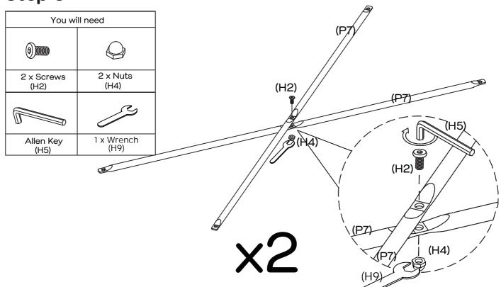
Secure Back Supports (P7×2) together as shown with 1 x Nut (H4) and 1 x Screw (H2) by tightening with the Allen Key (H5) and Wrench (H9). Repeat steps for the second set of Back Supports (P7×2).
