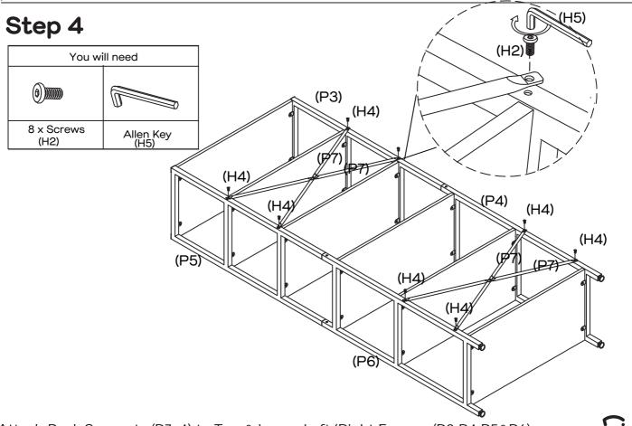
Attach Back Supports (P7x4) to Top & Lower Left/Right Frames (P3,P4,P5&P6) as shown with 8 x Screws (H2) by tightening with the Allen Key (H5).
