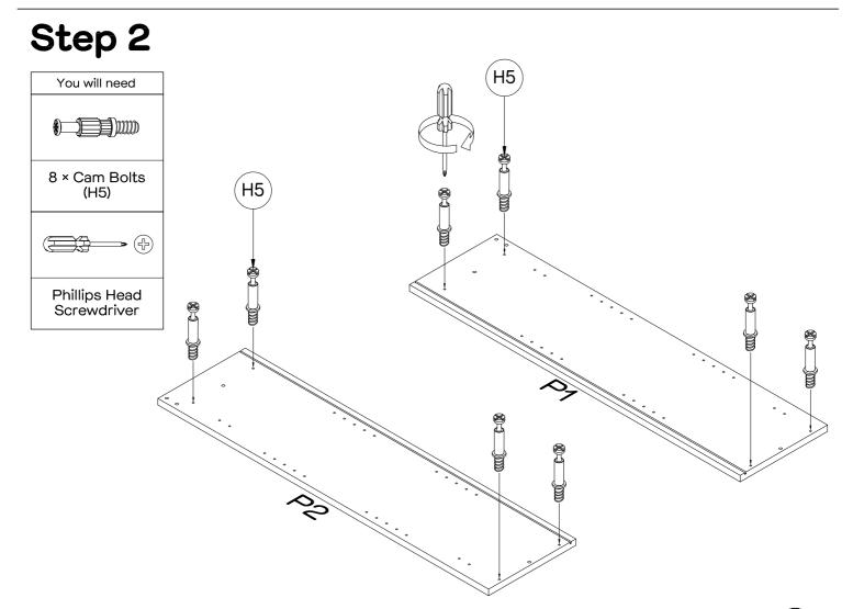
Secure  $4 \times Cam$  Bolts (H5) to Left Side Panel (P1) and  $4 \times Cam$  Bolts (H5) to Right Side Panel (P2) by tightening with the Phillips Head Screwdriver.
