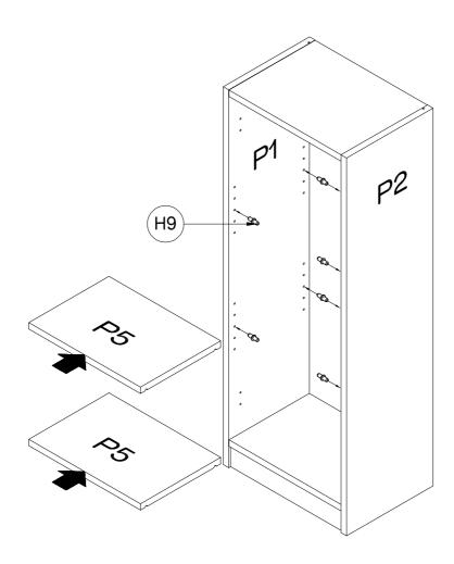
Insert 8 x Shelf Studs (H9) into the Left & Right Side Panels (P1&P2) at your preferred height. Place the Shelf Panels (P5x2) into the unit by resting each shelf on the shelf studs. Ensure each shelf is positioned securely.
