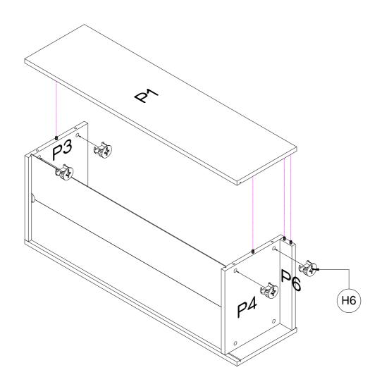
Insert 2 x Cam Nuts (H6) into Top Panel (P3) and 2 x Cam Nuts (H6) into Bottom Panel (P4) as shown. Rotate the cam nuts so the arrows point towards the incoming cam bolts. Secure the Left Side Panel (P1) to Top & Bottom Panels (P3&P4) by tightening cam nuts with a Phillips Head Screwdriver.
