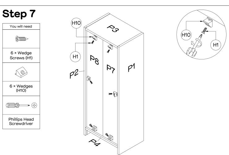
Insert 6 x Wedges (H10) into Top Panel (P3), Bottom Panel (P4) and Side Panels (P1&P2) as shown and use 6 x Wedge Screws (H1) to secure by tightening with the Phillips Head Screwdriver.
