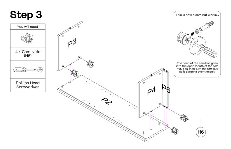
Insert 2 x Cam Nuts (H6) into Top Panel (P3) and 2 x Cam Nuts (H6) into Bottom Panel (P4) as shown. Rotate the cam nuts so the arrows point towards the incoming cam bolts. Secure the Right Side Panel (P2) to Top & Bottom Panels (P3&P4) by tightening cam nuts with a Phillips Head Screwdriver. Insert Front Panel (P6) into Right Side Panel (P2) as shown.
