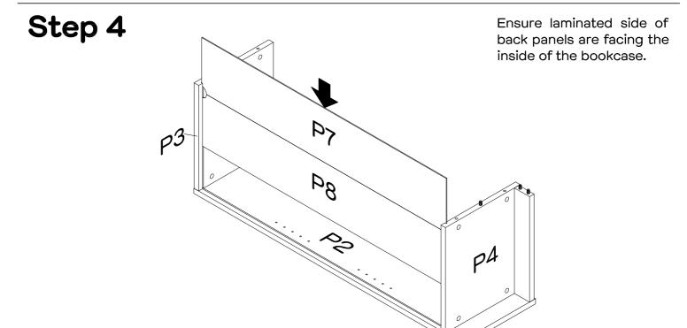
Slide Back Panels (P7&P8) into the grooves of Right Side Panel (P2) and Top & Bottom Panels (P3&P4) as shown.
