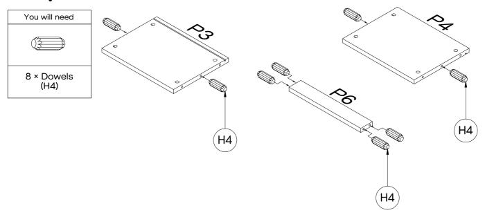
Insert 2 x Dowels (H4) into Top Panel (P3),  $2 \times 1$  Dowels (H4) into Bottom Panel (P4) and  $4 \times 1$  Dowels (H4) into Front Panel (P6).
